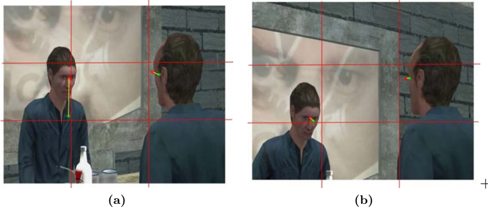
Figure 3.10 – The evaluation of a camera configuration w.r.t. frame composition is expressed as the Euclidian distances between on-screen actual positions (red) and desired positions (green) of characters eyes. The solving process seeks for minimizing these distances using a local search optimization process.
