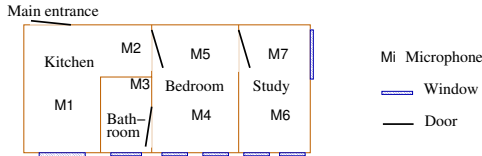
Figure 1: Position of the 7 microphones in the DOMUS Home
