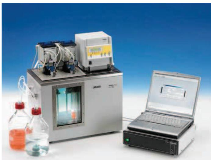
**Figure 15 :** Appareillage Lauda Proline PV 15
