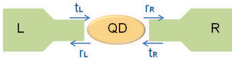
Figure 2.13: Schematics of the Landauer-Buttiker type of transmission model adopted by Man et al to explain the spin-dependent conductance in a MTJ containing a quantum dot.
