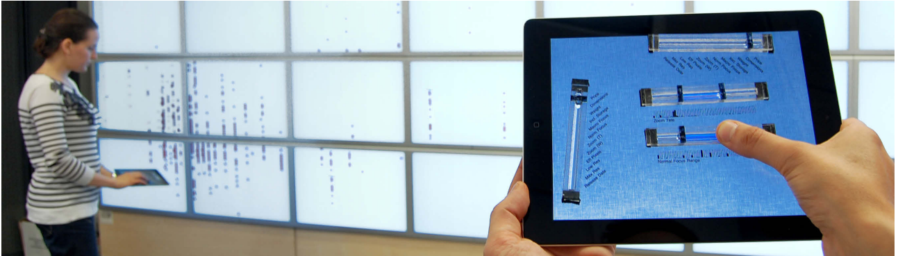
Figure 4.6: Example scenario for tangible remote controllers in a WSD environment. A scatterplot is displayed on the WSD and two users are controlling its parameters using their respective controllers.
