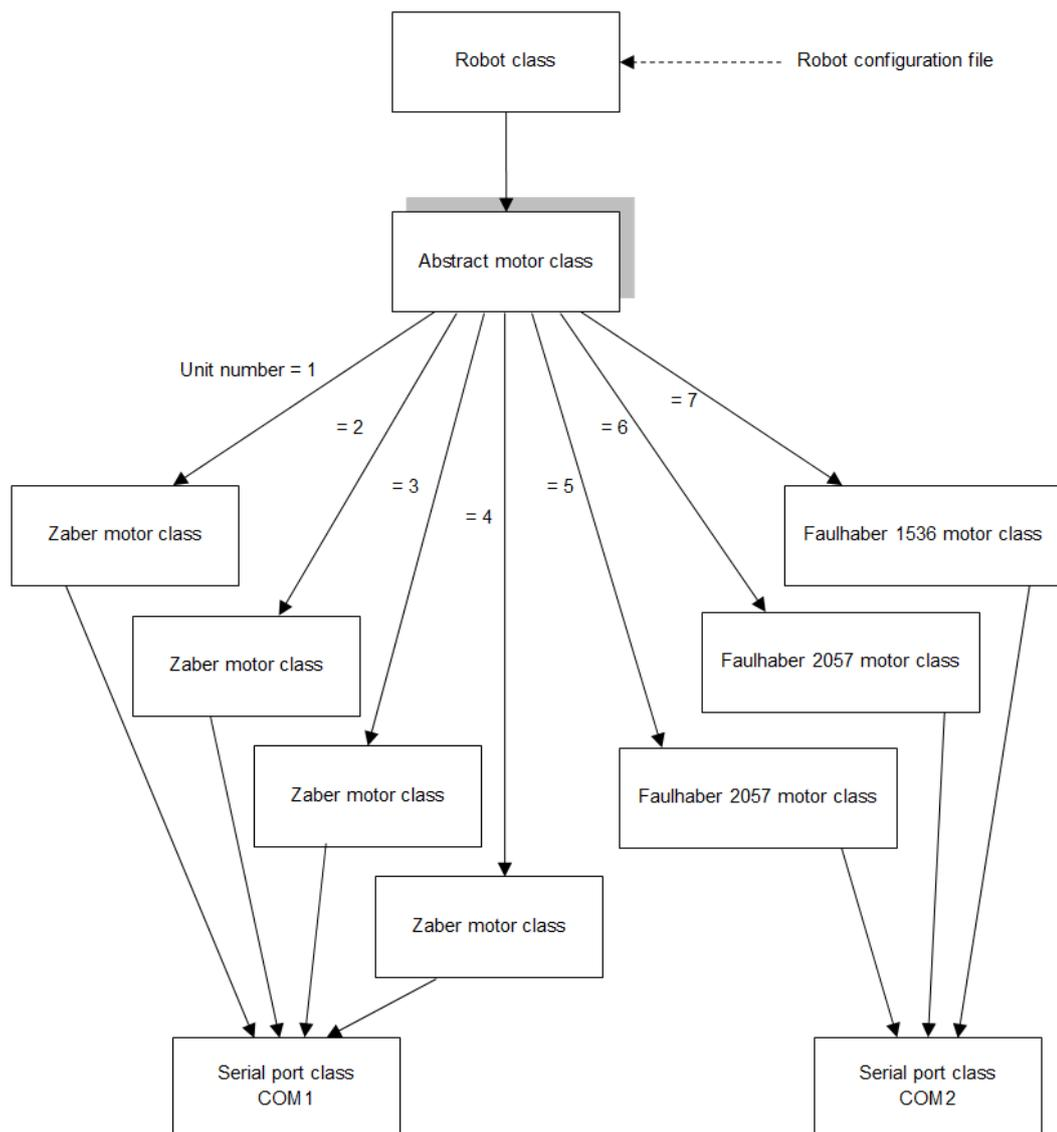
Figure 3-14: Block diagram describing the software design for controlling the PROSPER prototype. Each block represents an instance of a class. Arrows show the inheritance between classes.
