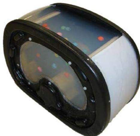
Figure 4-26: Photograph of the phantom constructed and used for the LPR system's accuracy tests.
