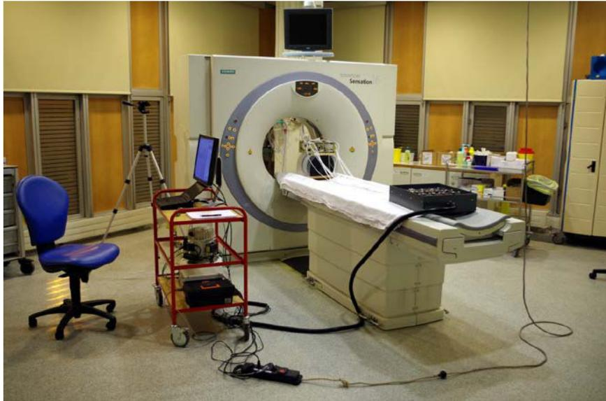
Figure 4-27: Photograph of the phantom experiment setup in the CT scanner room. The robot is placed over the phantom at the head of the scanner table. The motor box is placed at the feet of the scanner table. The work area, including control PC, control box and a compressor were placed within the imaging room in order to have a closer view of the robot motions during the experiments.
