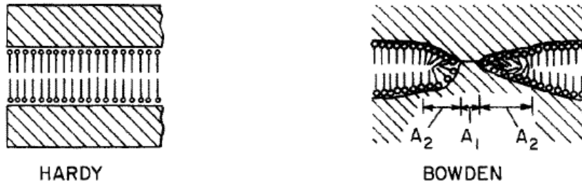
FIGURE 4: BOUNDARY LUBRICATION MODEL, HARDY: ADSORPTION OF MONOLAYER OF POLAR MOLECULES, BOWDEN: INTIMATE CONTACT OF SOLID SURFACES OCCURS [18]
