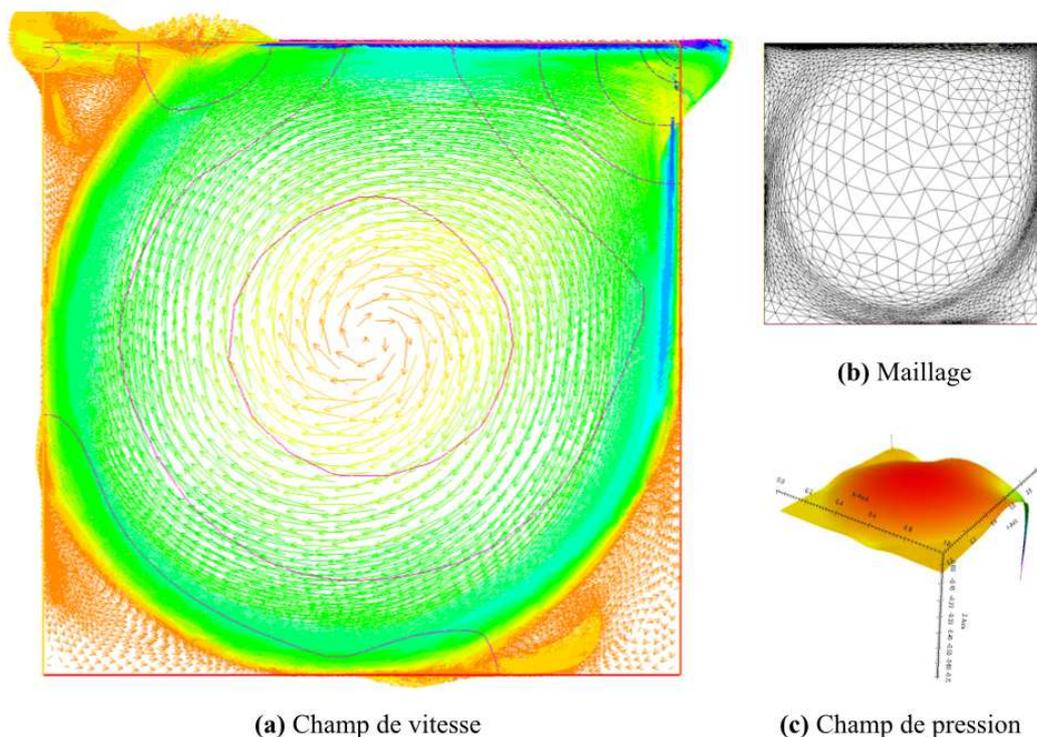
FIGURE 1.10: Fluide incompressible  $R_e = 10000$
