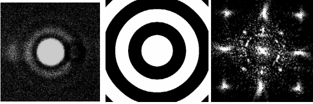
Fig. 16. PSF of the 0.8 mm reference pupil ( \gamma = 10 ) (right). From this PSF we constructed the sign mask (center). The white zones are uniform and equal to 1 and the black zones are equal to -1 . Multiplying I_- by this mask, the correction can be achieved (right) for this reference pupil.
