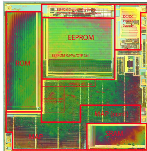
Figure 2.10 – Decapsulated smart card chip [IOA12].
