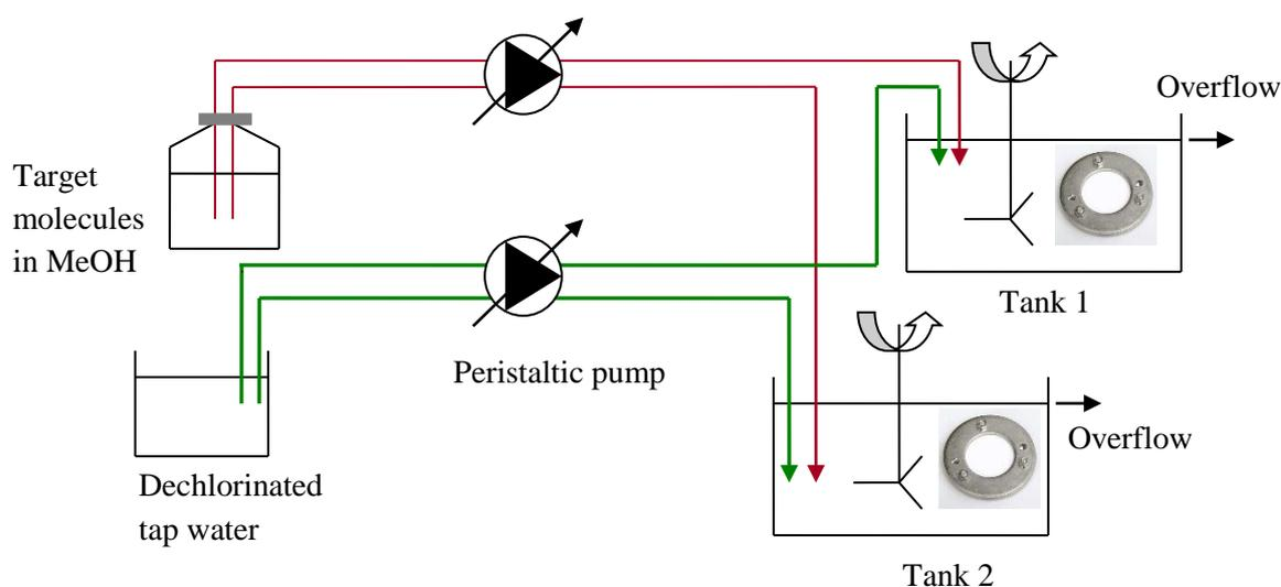
Figure 1 – Experimental design used for calibrations in the laboratory
