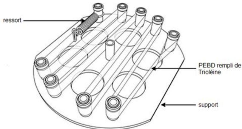
Figure 9 - Echantillonneur passif de type SPMD (Seethapathy et al. 2008)
