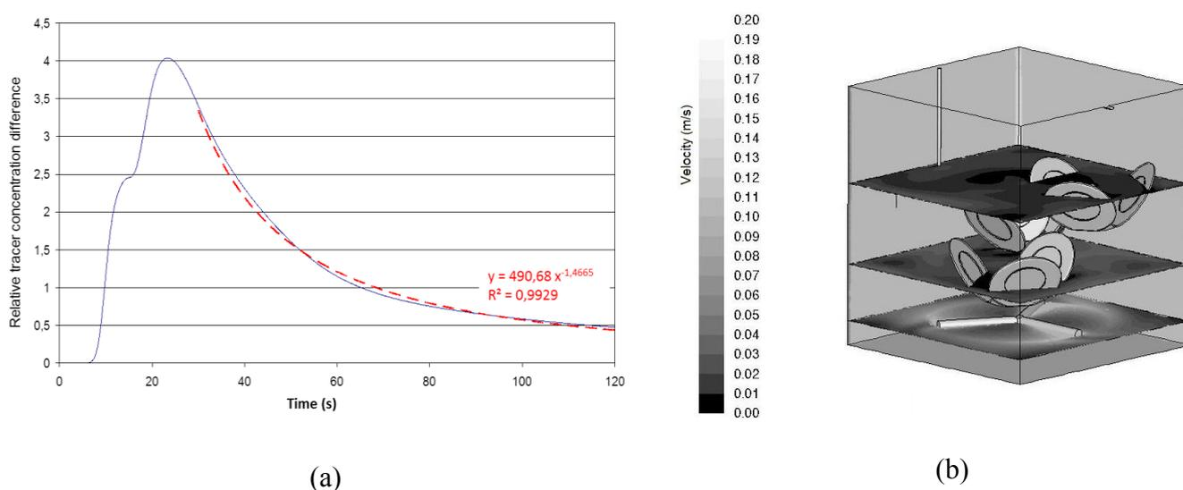
Figure 4. Maximal relative concentration difference between POCIS surfaces over the 120 first seconds (a) and representation of water flow rate ( $m \cdot s^{-1}$ ) in the exposure tank (b)
