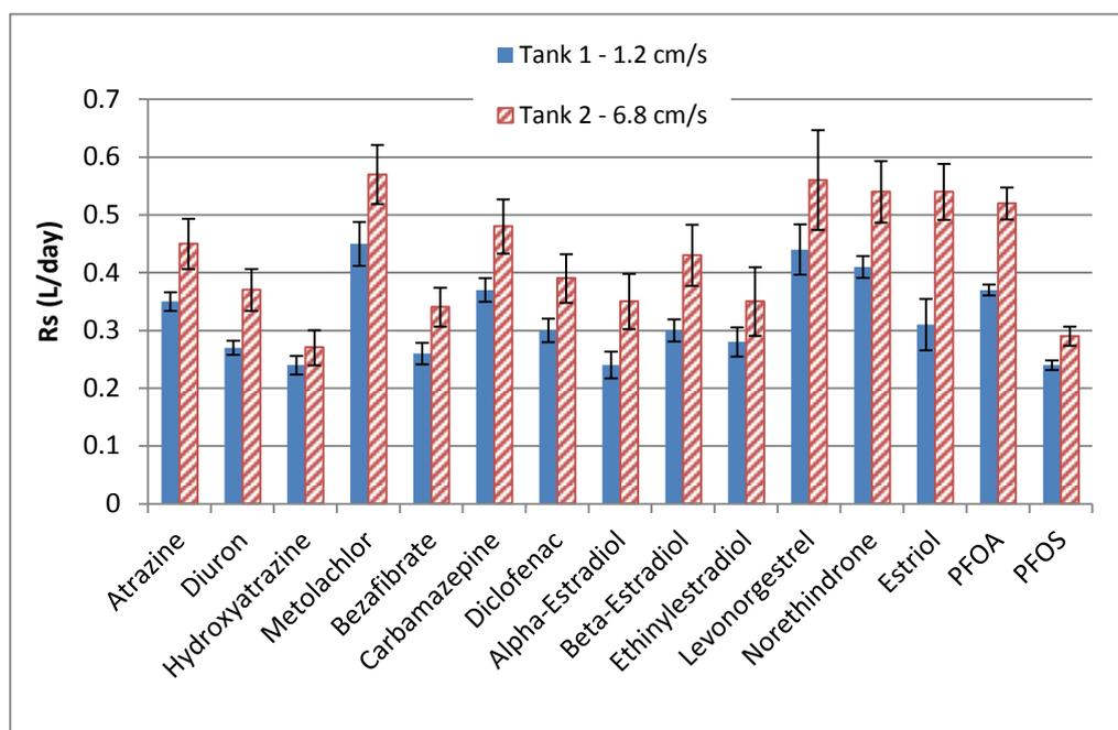
Figure 4 – POCIS sampling rates determined at two different water velocities
