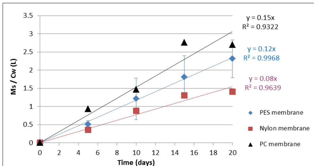
Figure 3 – Branched-PFOS accumulation in the POCIS with the three types of membranes (error bars indicate standard deviations obtained for PES membranes,  $n = 3$ )
