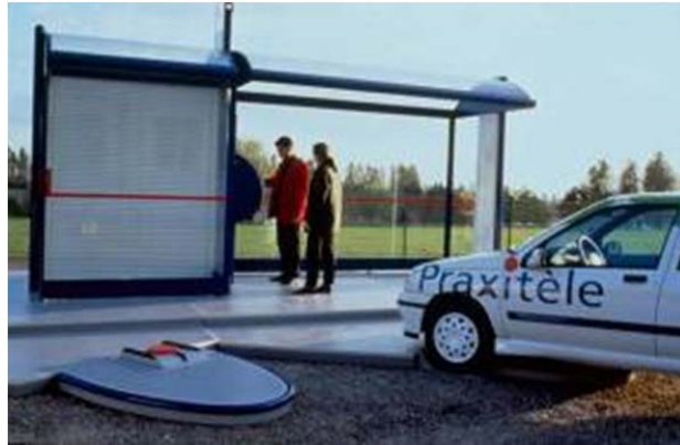
Fig. 0.2: PRAXITELE Wireless EV battery charging using electric billing payment [1]
