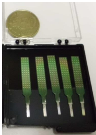
Figure 41 – MEA fourchettes sur silicium
