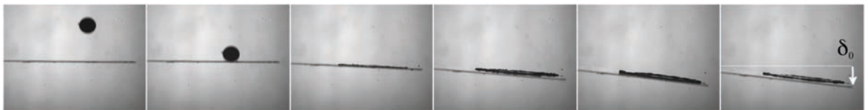
Figure V.7 – Galinstan drop of radius R = 1.25 mm and speed V = 4 m/s hitting the edge of a thin glass plate. Images are separated by 1 ms and only show 1/3 of the lamella. We denote \delta_0 as the maximum plate deflection after impact.
