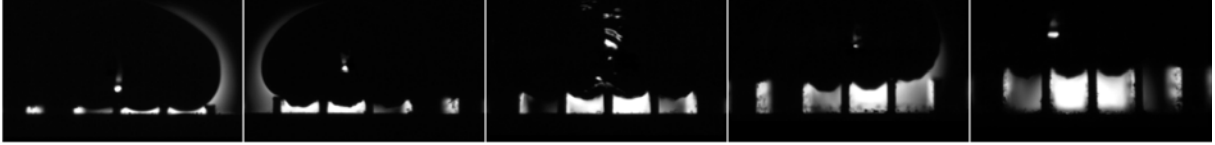
Figure I.25 – Side zoom view of a Leidenfrost puddle drop sitting on crenels of fixed width W = 1 \text{ mm} and wall thickness \lambda = 0.2 \text{ mm} . Depth H from left to right is 200 \mu\text{m} , 400 \mu\text{m} , 600 \mu\text{m} , 800 \mu\text{m} and 1200 \mu\text{m} . On the left image, where H = 200 \mu\text{m} < h , \epsilon is smaller due to the vapor cushion overpressure.
