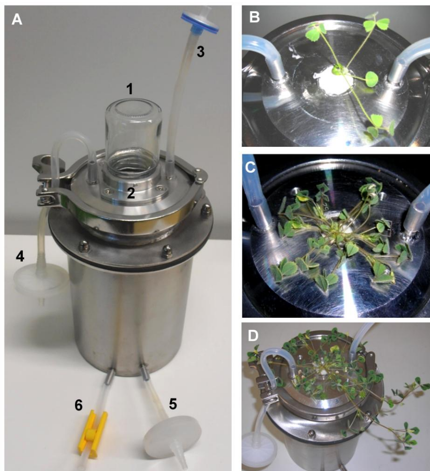
Figure 1.S1 Description and illustration of a gnotobiotic pot. Gnotobiotic pot (A) made for the experiment allowing the growth of Medicago truncatula in microbiologically controlled conditions because of a glass pot (1) fixed to the cover with a plate (2) during 15 days at the beginning of growth. After this date, glass pot was removed and silicone was disposed around the hypocotyl (B). The plant was watered through a 0.2 \mu\text{m} filter (3). Air circulation is done through two air filters (4,5). The water outlet was controlled manually with a clamp (6). Figures (C) and (D) show more advanced developmental stage, corresponding to 35 days without and with the strain respectively, in \text{CO}_2 ambient conditions.
