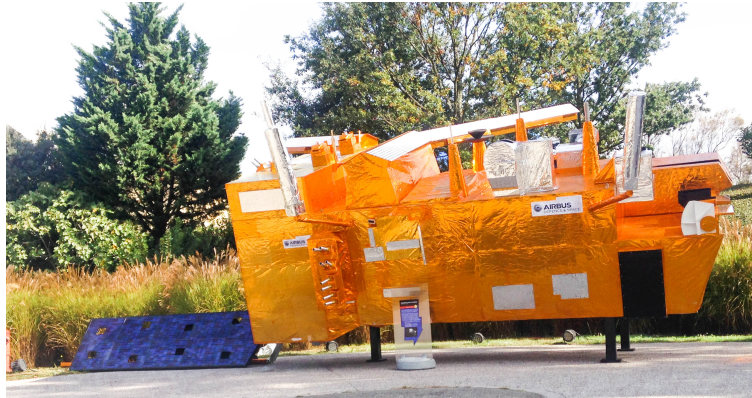
Figure 3.1: 1:1 model of the MetOp Satellite.
