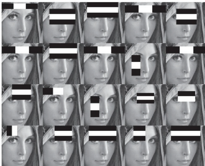
Figure 2.14: Haar-like features extracted from different position and different scale on the face image.
