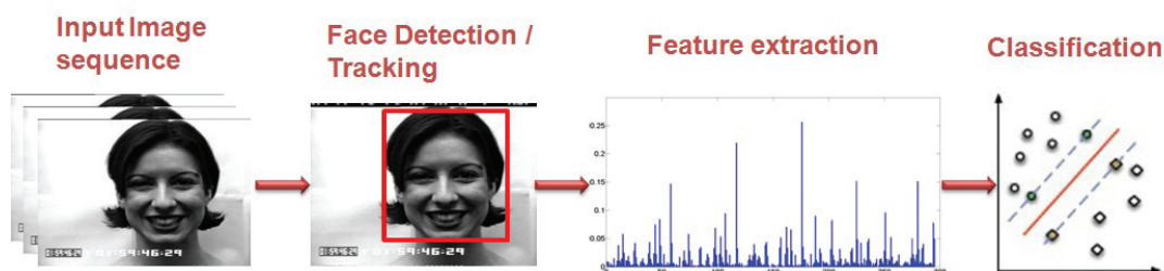
Figure 2.8: Automatic facial expression recognition system pipeline.
