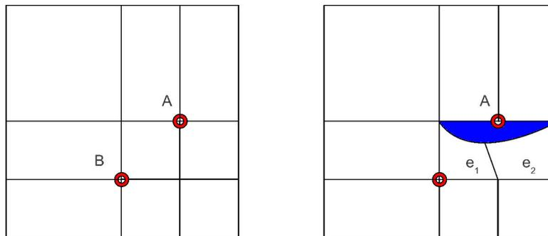
Figure 5.3: *Problem of discontinuity in the method of introducing irregular nodes at the edge centers of a very simple mesh. Suppose points A and B are points where irregular nodes have been placed. If for some reason, the elements  $e_1$  and  $e_2$  are forced to bend their top edges, then the result is an area that is totally empty (blue area in Figure 5.3).*
