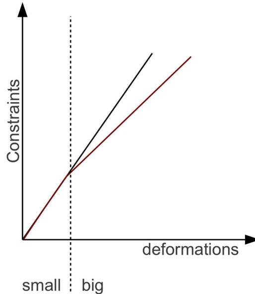
Figure 3.2: *Elastic behaviour of a material. The linear approximation is valid for small deformations. Depending on the application and accuracy required, the limit between small and big requirement in deformation may vary between 5%-20%.*
