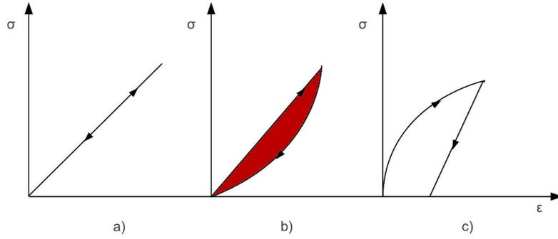
Figure 3.3: *Stress-Strain curves for a purely elastic material (a), a viscoelastic material (b) and a plastic material (c). The red area in (b) is a hysteresis loop and shows the amount of energy lost in a loading and unloading cycle. The material in (c) suffers plastic deformation and fails to return to its rest shape.*
