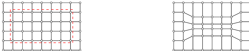
(a) A simple grid of quadrangular elements with the region to refine in red. (b) Nodes are moved to follow the phenomenon in the selected region.
