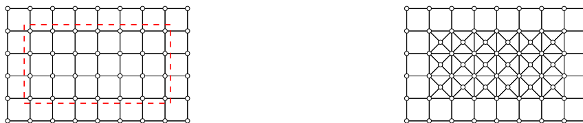
(a) A simple grid of quadrangular elements with the region to refine in red. (b) The area has been remeshed with triangles.
