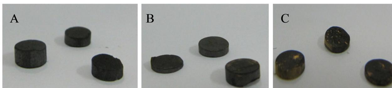
**Figure II.4.4.** Morphologie des disques de carbones poreux C-HIPE<sub>(60Carb)</sub> (A), 5-Au@C-HIPE<sub>(60Carb)</sub> (B), 15-Au@C-HIPE<sub>(60Carb)</sub> (C).
