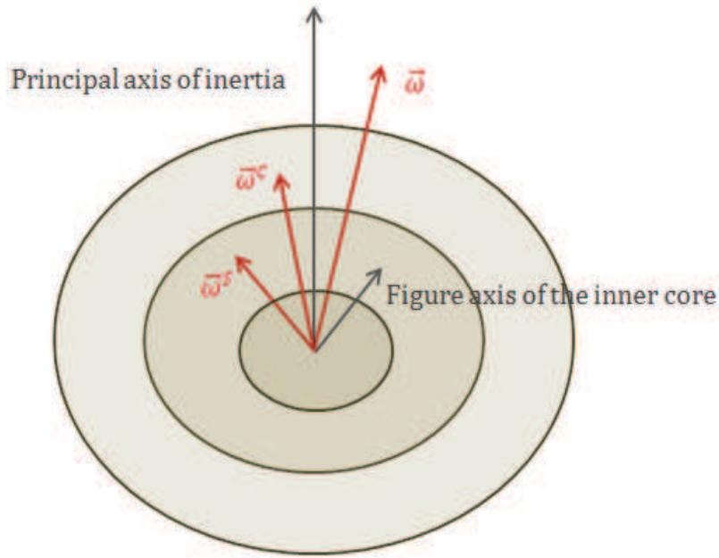
**Fig. 6.2:** Diagram of the whole-Earth axis of rotation, the axis of rotation of the inner core, the angular velocity of the mantle and the differential rotation of the outer and inner core with respect to the mantle.
