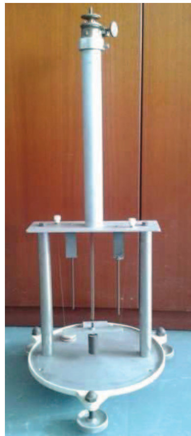
Fig. 2.2.4: Simplified scheme of a bifilar gravimeter, after Melchior (1966), and picture of bifilar gravimeter owned by IPGS.
