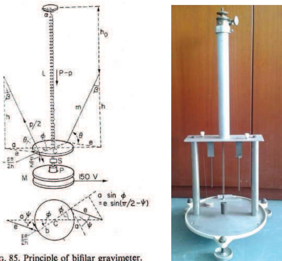
FIG. 85. Principle of bifilar gravimeter.
