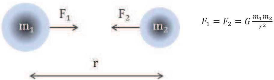
**Fig. 2.1.1:** Diagram of Newton's law of gravity.
