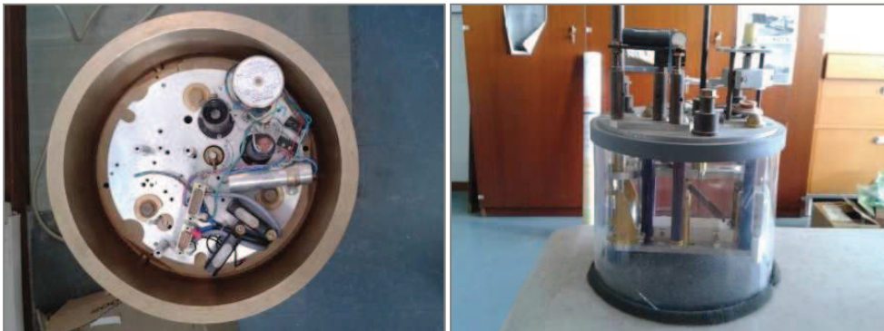
Fig. 3.3: North American 138 which was installed at the Seismological Observatory of Strasbourg in consecutive periods from 1955 until 1967.
