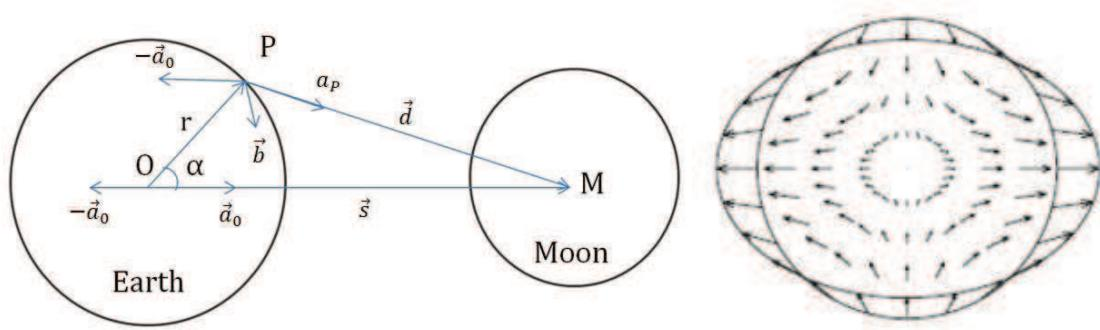
**Fig. 2.1.2:** Tidal forcing. The left plot shows the geometry of the problem for computing the tidal force at a point  $P$  on the Earth, given an external body  $M$  (Moon). The right plot shows the field of forces (accelerations) for the actual Earth–Moon separation. The elliptical line shows the equipotential surface under tidal forcing, greatly exaggerated (adapted from Agnew, 2007).
