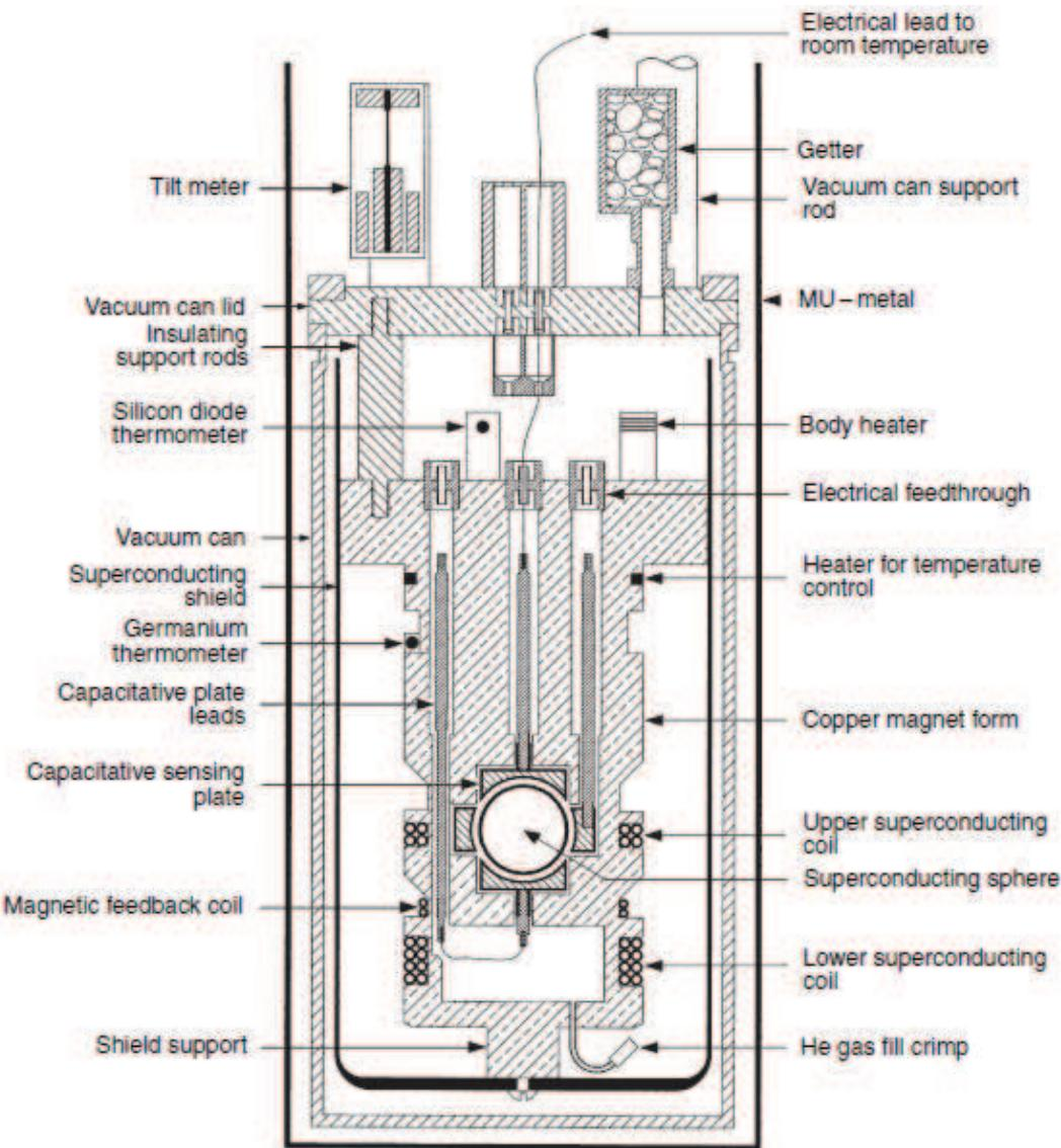
**Fig. 2.2.7:** Main components of the superconducting gravimeter dewar and sensor (extracted from GWR website, <http://www.gwrinstruments.com>).
