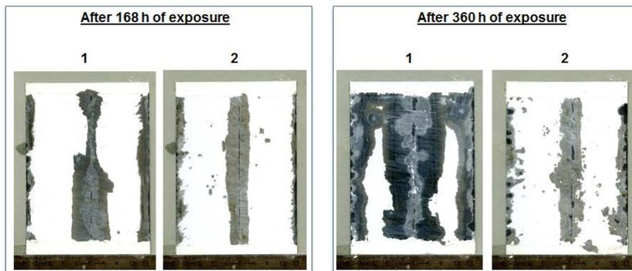
Figure 7.1: Salt spray test of galvanized steel coated with (2) and without (1) LDH/MoO<sub>4</sub><sup>2-</sup> fillers after 168 and 360 hours of exposure
