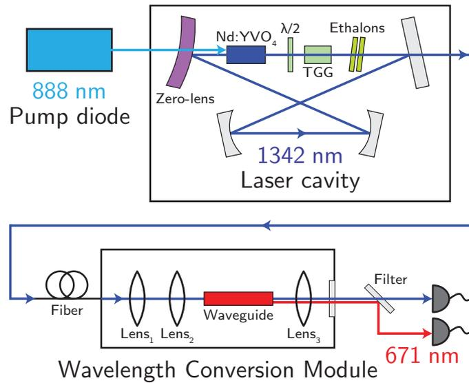
Fig. 3. (Color online) Schematic view of the frequency doubling setup. Shown are the IR laser cavity and the wavelength conversion module. The pump diode output is focused in the Nd:YVO<sub>4</sub> laser crystal inside the laser cavity, which also contains a Faraday rotator and a  $\lambda/2$ -waveplate for unidirectional oscillation and two etalons for frequency selection. The wavelength conversion module includes a ppZnO:LN nonlinear waveguide for second-harmonic generation.
