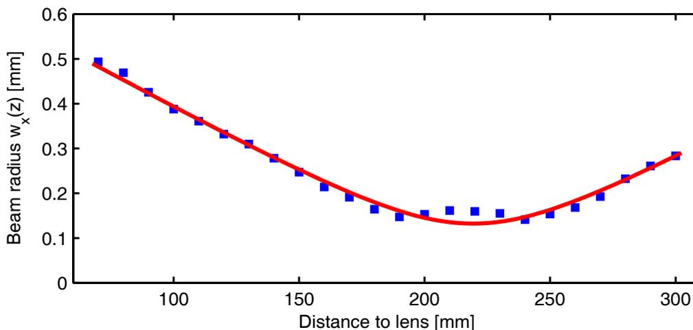
**Figure 5.17:** Beam quality measurement performed on the horizontal direction of the laser output beam. The  $M^2$  fit yields a value compatible to  $M^2 = 1$ , or pure Gaussian (TEM<sub>00</sub>) output.
