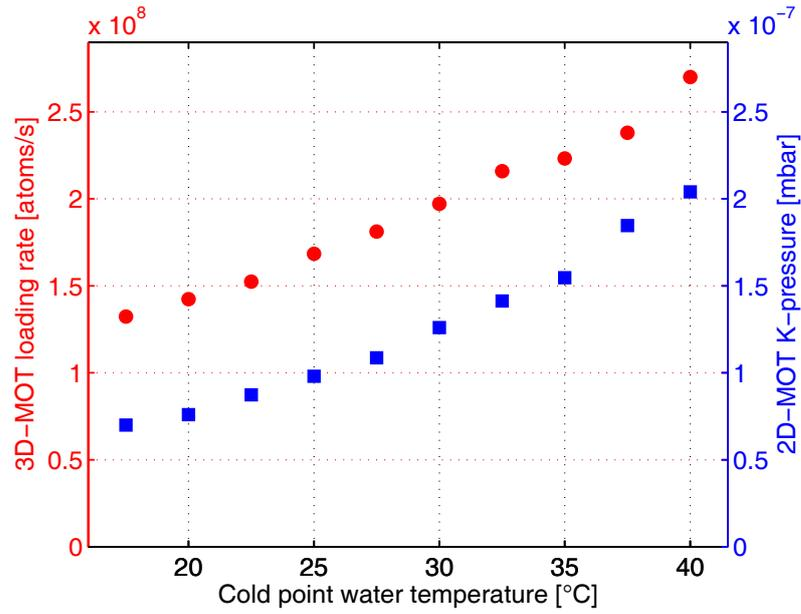
**Figure 2.10:**  $^{40}\text{K}$  3D-MOT loading rate (red circles) and total potassium 2D-MOT pressure (blue squares) as a functions of the cold point water temperature. The pressure is deduced from the absorption of a weak probe beam which is resonant with the  $D_2$  transition of  $^{39}\text{K}$  and passes through the 2D-MOT cell.
