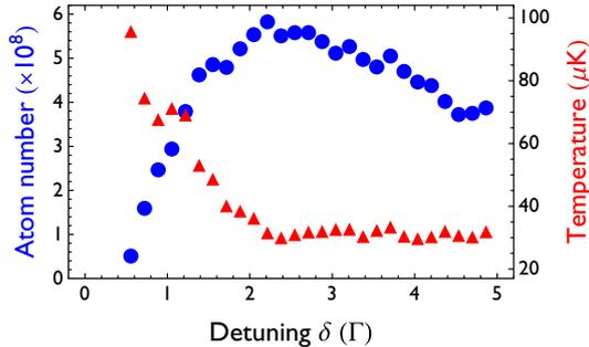
Fig. 7: (Color online) Number of atoms captured in the  $D_1$  molasses (circles) and their temperature (triangles) for the dynamic 8 ms cooling sequence as a function of the detuning  $\delta$ . The number of atoms in the compressed MOT was  $6 \times 10^8$ .
