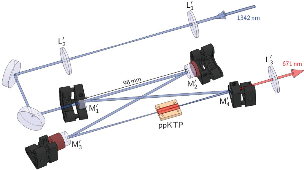
Fig. 7. (Color online) Scheme of the doubling cavity setup comprising the four mirrors  $M'_{1-4}$  and the ppKTP nonlinear crystal. The light is coupled to the Gaussian cavity eigenmode using lenses  $L'_{1,2}$ , whereas  $L'_3$  collimates the SH output. The crystal mount is depicted sectioned to improve visibility and the IR (SH) beam is illustrated in blue (red). The distance  $M'_3$ – $M'_4$  is 156 mm.
