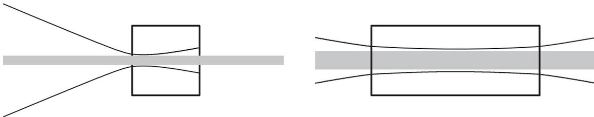
**Figure 5.8:** Tight pump beam focusing in a short crystal that is end-pumped at 808 nm (left) and less tight focusing in a longer crystal that is end-pumped at 888 nm (right), as published in [189]. The laser mode is illustrated in gray.
