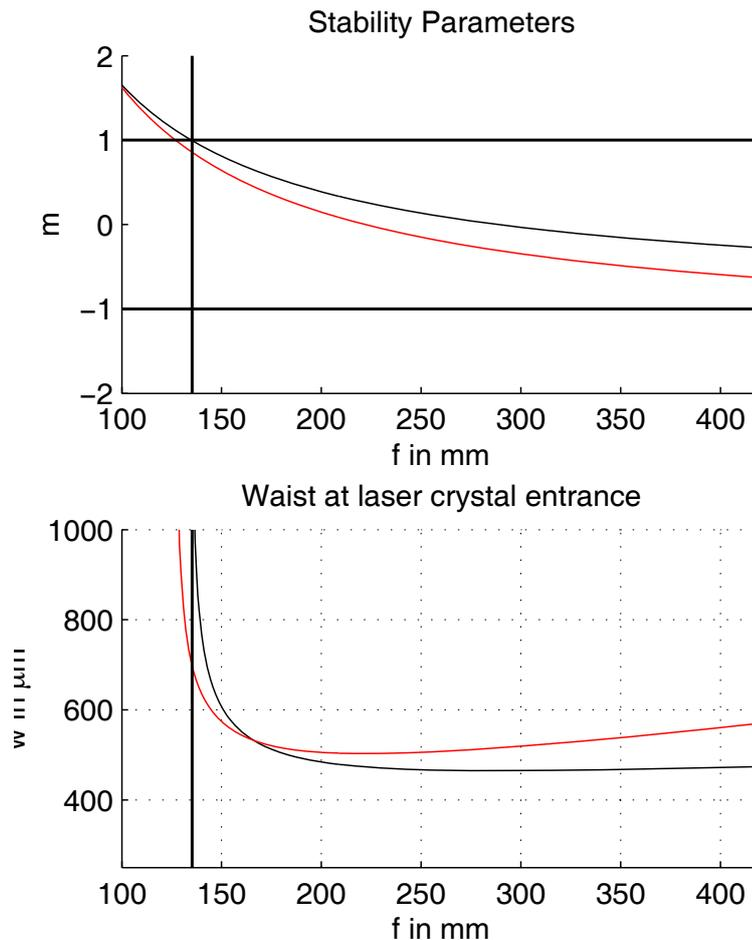
**Figure 5.11:** The stability diagram (upper panel, see Equation (5.14)) and the mode sizes (lower panel) in the laser crystal as a function of the thermal lens focal length  $f_{\text{th}}$ . The black (red) lines denote the horizontal (vertical) direction. The vertical line indicates the limit of cavity stability. The resonator remains stable down to  $f_{\text{th,min}} = 135 \text{ mm}$ .
