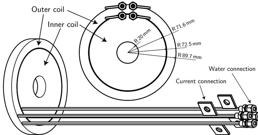
**Figure 2.13:** Technical drawing of the quadrupole coils which also serve as Feshbach coils (from [148]). They consist of two concentric coil pairs, an inner one and an outer one, both made of hollow copper wire impregnated in epoxy. The inner coils generate in particular the magnetic field for the optically plugged magnetic trap. They are placed at a distance of 17.5 mm from the trap center and create an axial magnetic field gradient of 2.51 G/cm A.
