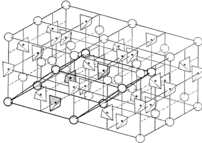
**Figure 5.3:** Crystal structure of YVO<sub>4</sub>, which is of the tetragonal zircon type, from [190]. The tetrahedra represent the VO<sub>4</sub><sup>3-</sup> ions, balls are Y<sup>3+</sup> ions. The unit cell is marked in bold lines.
