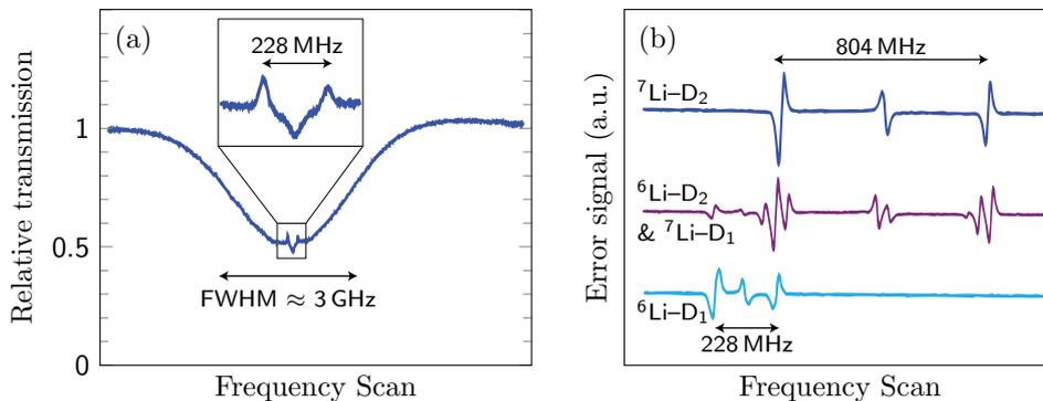
**Figure 6.11:** Doppler-free saturated absorption spectroscopy of the lithium D-lines. (a) Sample scan over the entire  ${}^6\text{Li D}_1$  Doppler-broadened absorption peak. The inset shows the sub-Doppler features. Similar spectra are obtained for all lithium D lines. (b) Error signals of all lithium D line transitions, generated by phase modulation spectroscopy. These signals provide an excellent reference for frequency-locking of the laser.
