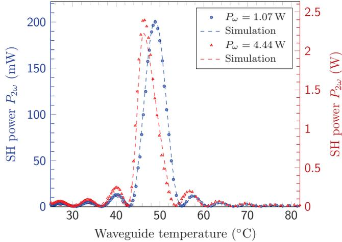
Fig. 4. (Color online) SH power as a function of the waveguide mount temperature  $T_{\text{mount}}$  at the fundamental IR pump power  $P_{\omega} = 1.07$  W and  $P_{\omega} = 4.44$  W coupled to the waveguide. Shown are the measured data points and the simulation results of our fitted model (dashed lines).
