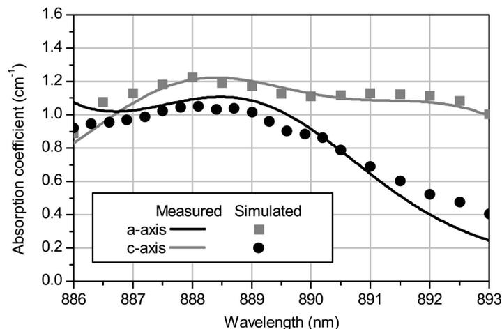
**Figure 5.7:** Theoretical curve for the convolution of the absorption spectrum with a 3.5 nm wide (FWHM) gaussian diode laser spectrum as well as experimental values for the effective absorption coefficient measured for a real 3.5 nm wide diode as a function of the center wavelength (from [193]).
