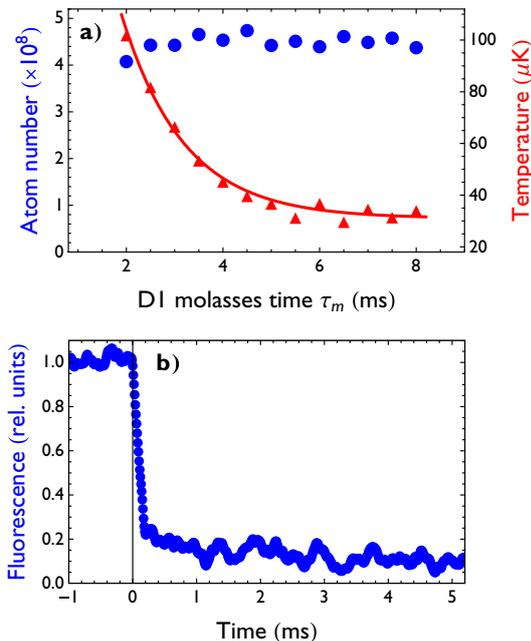
Fig. 4: (Color online) a) Number of atoms captured in the  $D_1$  molasses (circles) and their temperature (triangles) as a function of molasses duration. The number of atoms in the compressed MOT was  $4.5 \times 10^8$ . b) Measured fluorescence during the MOT and the  $D_1$  molasses phase. Both experiments were performed with  $I_{\text{cool}} = 14I_{\text{sat}}$ ,  $\delta = 2.3\Gamma$  and  $I_{\text{repump}} = I_{\text{cool}}/8$ .
