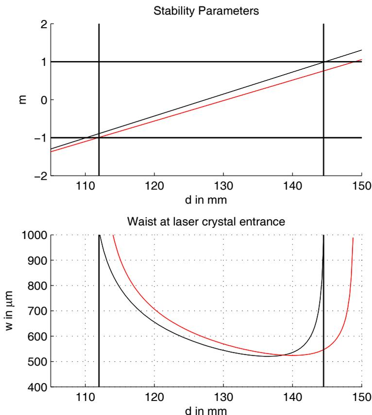
**Figure 5.12:** (Upper Panel) The stability parameters of the laser cavity as a function of the distance  $d_{\text{cu}}$  between the curved mirrors  $M_3$  and  $M_4$ . The thermal focal length is fixed to 170 mm. (Upper Panel) The mode sizes in the laser crystal  $w_{h(v)}$ , the black (red) lines denoting the horizontal (vertical) direction, whereas the vertical lines indicate the range of stability.
