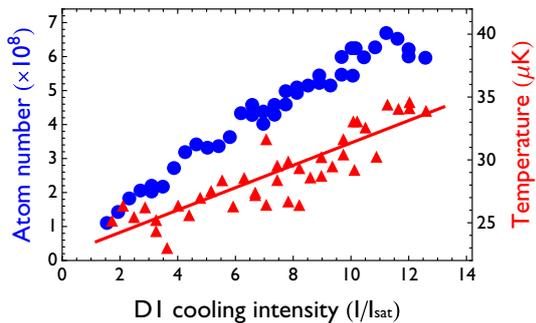
Fig. 5: (Color online) Number of atoms captured in the  $D_1$  molasses (circles) and their temperature (triangles) as a function of the  $D_1$  cooling beam intensity for  $\delta = 2.3\Gamma$  and  $I_{\text{repump}} = I_{\text{cool}}/8$ . The number of atoms in the compressed MOT was  $6.5 \times 10^8$  and the capture efficiency reaches  $\sim 100\%$  for  $I \geq 11I_{\text{sat}}$ .
