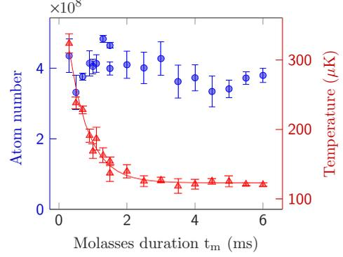
FIG. 8. (Color online) Number of atoms captured in the  ${}^6\text{Li}$   $D_1$  molasses (circles) and their temperature (triangles) as functions of the molasses duration, with a  $1/e$  cooling time constant  $\tau_{\text{cool}} = 0.6 \text{ ms}$ . The number of atoms in the compressed MOT is  $8 \times 10^8$ .
