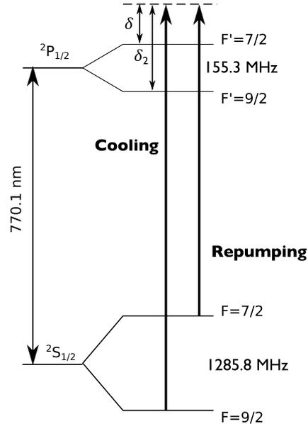
Fig. 2: Level scheme for the  $D_1$  transition of  $^{40}\text{K}$  and transitions used for gray-molasses cooling. The laser detuning from the cooling/repumping transitions is  $\delta$  and the detuning from the off-resonant excited hyperfine state  $F' = 9/2$  is  $\delta_2$  (see text).
