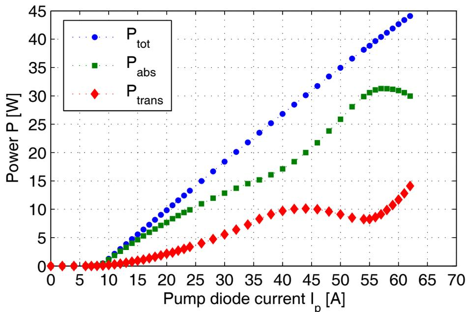
**Figure 5.14:** Absorption of the pump light ( $w_{\text{pump}} = 970 \mu\text{m}$ ) by the 25 mm long Nd:YVO<sub>4</sub> crystal with 0.5 at. % doping. Shown are the total power incident on the laser crystal  $P_{\text{tot}}$ , the transmitted power  $P_{\text{trans}}$  and the absorbed pump power  $P_{\text{abs}}$  as a function of the current  $I_p$  passing through the pump diode stack at a cooling water temperature set to 4°C. Saturation of pump light absorption sets in at  $I_p = 57$  A.
