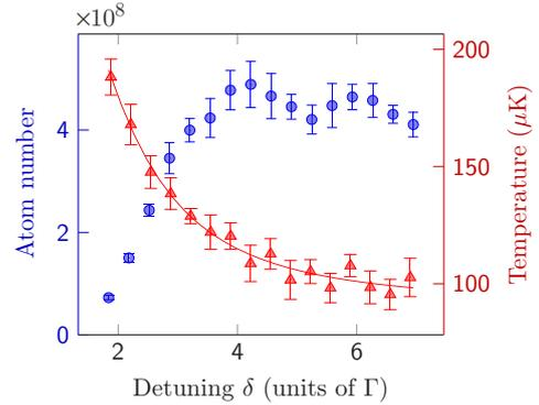
FIG. 9. (Color online) Number of atoms captured in the  ${}^6\text{Li}$   $D_1$  molasses (circles) and their temperature (triangles) after a 3-ms capture phase at a high intensity,  $I_{\text{cool}} = 14.6I_{\text{sat}}$ , as functions of the global detuning  $\delta = \delta_{\text{cool}} = \delta_{\text{rep}}$ . The number of atoms in the compressed MOT is  $8 \times 10^8$ .
