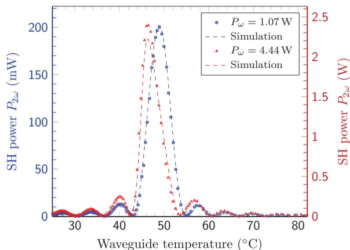
**Figure 6.13:** SH power as a function of the waveguide mount temperature  $T_{\text{mount}}$  at the fundamental IR pump power  $P_{\omega} = 1.07$  W and  $P_{\omega} = 4.44$  W coupled to the waveguide. Shown are the measured data points and the simulation results of our fitted model (dashed lines).
