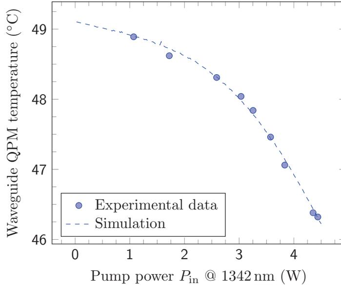
**Figure 6.14:** Optimal crystal mount temperature  $T_{\text{mount,opt}}$  during SHG process in dependence of the fundamental IR pump power  $P_{\omega}$  coupled to the waveguide. The crystal mount temperature is adjusted for every pump power value in order to maximize the corresponding SH power.
