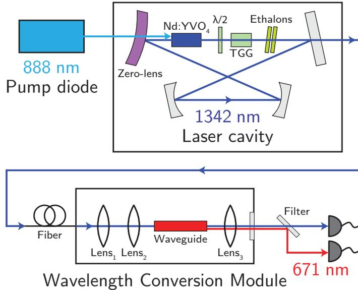
**Figure 6.12:** Schematic view of the frequency doubling setup. Shown are the IR laser cavity and the wavelength conversion module. The pump diode output is focused in the Nd:YVO<sub>4</sub> laser crystal inside the laser cavity, which also contains a Faraday rotator and a  $\lambda/2$ -waveplate for unidirectional oscillation and two etalons for frequency selection. The wavelength conversion module includes a ppZnO:LN nonlinear waveguide for second-harmonic generation.
