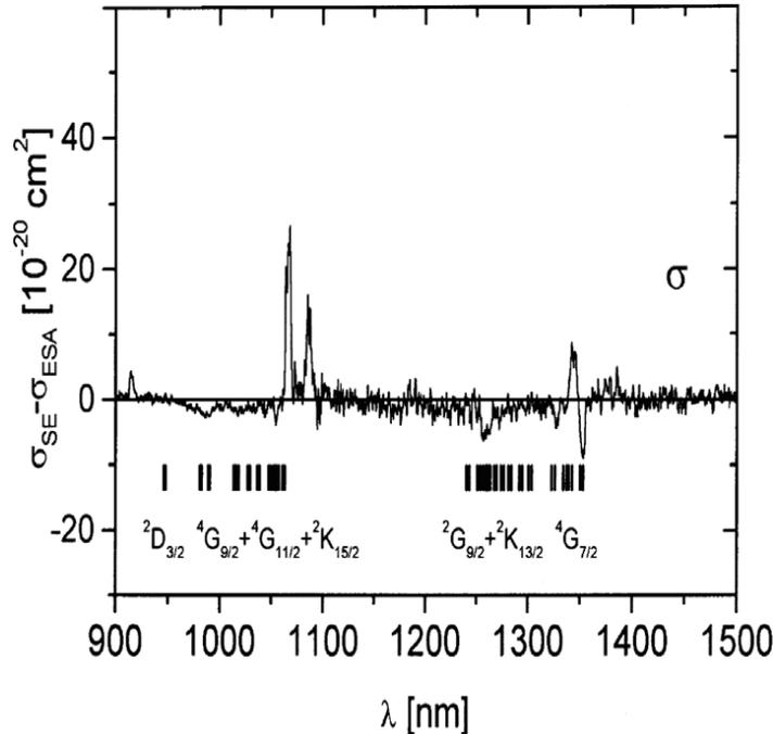
**Figure 5.4:** Emission spectrum of Nd:YVO<sub>4</sub> measured for the c-axis with a spectral resolution of  $2.5\ \text{nm}$  (from [199]). It exhibits two noticeable features around  $1064\ \text{nm}$  and at  $1342\ \text{nm}$ .
