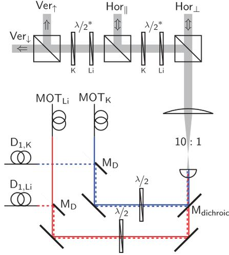
FIG. 7. (Color online) Optical scheme of the  $D_1$  molasses. The 3D MOT light and the  $D_1$  cooling light are superposed using a D-shaped mirror ( $M_D$ ). Afterwards a dichroic mirror ( $M_{\text{dichroic}}$ ) combines the lithium and potassium light, which is subsequently expanded and distributed to the three perpendicular axes of the 3D MOT.
