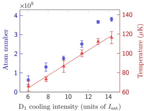
FIG. 10. (Color online) Number of atoms captured in the  ${}^6\text{Li}$   $D_1$  molasses (circles) and their temperature (triangles) as functions of the  $D_1$  cooling beam intensity for  $\delta_{\text{cool}} = 4 \Gamma$  and  $I_{\text{rep}} = I_{\text{cool}}/20$ . The number of atoms in the compressed MOT is  $8 \times 10^8$ . The atom number (temperature) increases linearly with a slope of  $4 \times 10^7$  atoms/ $I_{\text{sat}}$  ( $6.5 \mu\text{K}/I_{\text{sat}}$ ).
