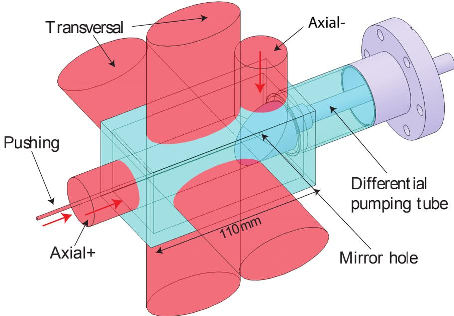
**Figure 2.8:** Scheme of the  $^{40}\text{K}$  2D-MOT and illustration of the light beams. The elliptic beams transversally cool the atoms. The alignment of the axial molasses beam pair is provided by a 45°-angled mirror placed inside the vacuum chamber. The pushing beam axially out-couples an atomic beam through the mirror hole. The optimal beam parameters are given in Table 2.2.
