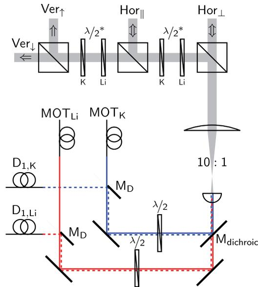
**Figure 2.12:** Optical scheme for the 3D-MOT and  $D_1$ -molasses beams, as presented in [148]. A D-shaped mirror ( $M_D$ ) nearly superposes the 3D-MOT light and the  $D_1$  molasses light for both atomic species. Subsequently, the lithium- and potassium light is combined at dichroic mirror ( $M_{\text{dichroic}}$ ). The resulting beam is finally expanded and distributed to three perpendicular axes forming the 3D-MOT.
