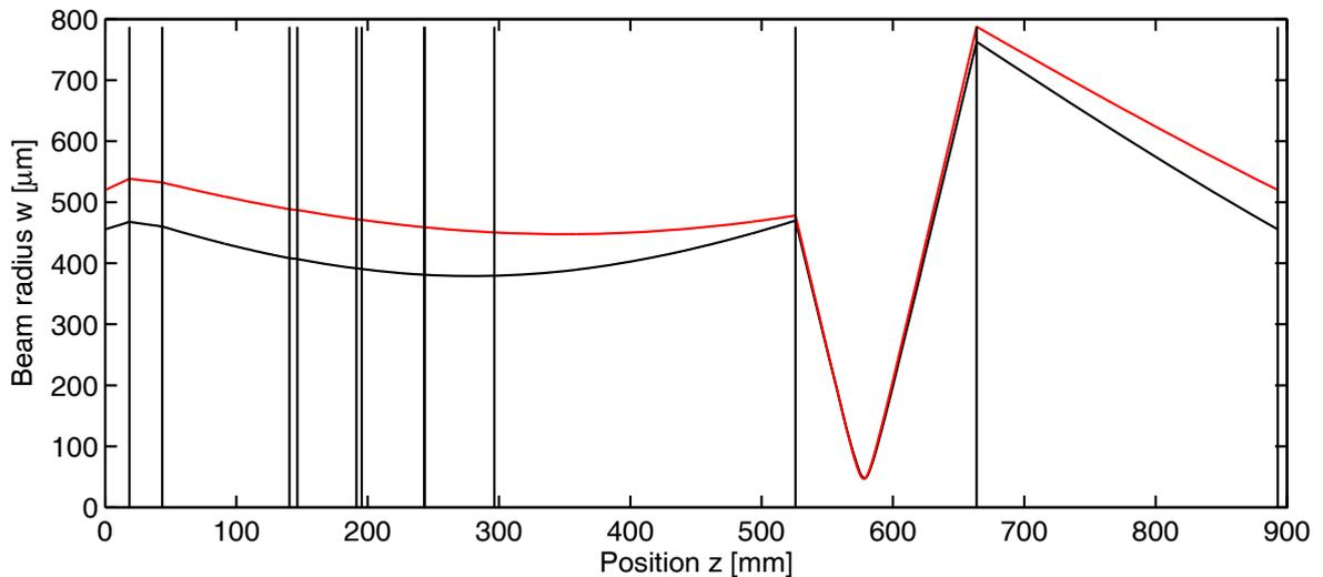
**Figure 5.19:** The eigenmode of the laser resonator. The horizontal (black) and the vertical (red) widths of the laser beam mode are shown as a function of the position inside the cavity. The vertical lines indicate the position of optical surfaces related to intra-cavity elements.  $z = 0$  corresponds to the position of the convex pump coupler ( $M_1$ ), and the sense of propagation is directed towards the output coupler ( $M_2$ ), which is located at 297 mm.
