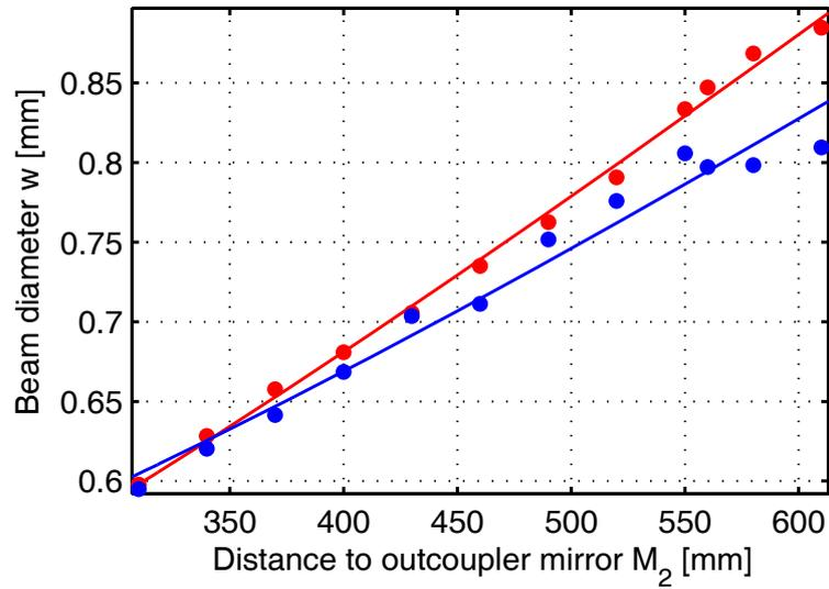
**Figure 5.18:** Measurement of the beam parameters (red/blue: horizontal<sub>x</sub>/vertical<sub>y</sub> waist) of the laser output beam. The fits assume  $M^2 = 1$ . This measurement is needed to calculate the necessary coupling optics for mode-matching the enhancement doubling cavity or the waveguide fiber. The ellipticity and astigmatism of the beam can in principle be corrected by cylindrical lenses.
