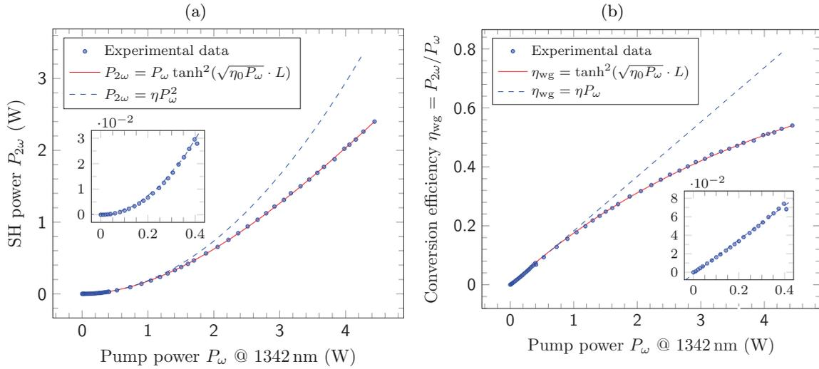
**Figure 6.15:** SH power output (a) and conversion efficiency (b) versus fundamental IR pump power coupled to the waveguide. The crystal mount temperature is adjusted for every pump power value as presented in Figure 6.14.
