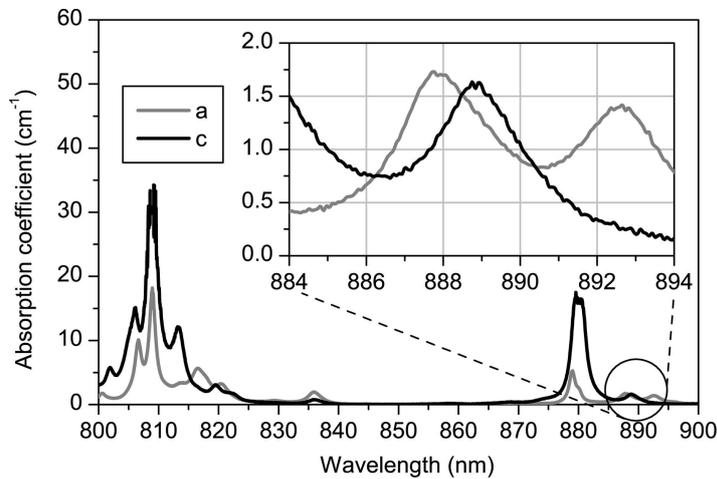
**Figure 5.6:** Absorption spectrum of Nd:YVO<sub>4</sub> (1 at.% doping) for light polarized parallel to the a- and c-axis in the wavelength range from 800 nm to 900 nm (from [193]). The material features several absorption bands at 808 nm, 880 nm and 888 nm, the latter being almost polarization-independent.
