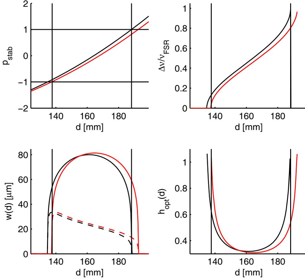
**Figure 6.2:** Several parameters of the doubling cavity as a function of the distance  $d$  between the two curved mirrors  $M'_3$  and  $M'_4$ . Black (red) lines indicate the horizontal (vertical) direction in the setup.
