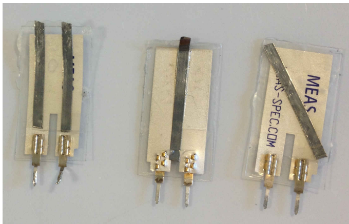
Figure 3.13: Different geometries of NiTiCu ribbons glued onto LDT-0 components.
