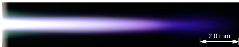
**Figure 2.1:** Photograph of the plasma jet visible effluent operating with 3.0 slm Ar. Exposure time of 0.25 s,  $f \setminus 7.1$ , 100 ISO.
