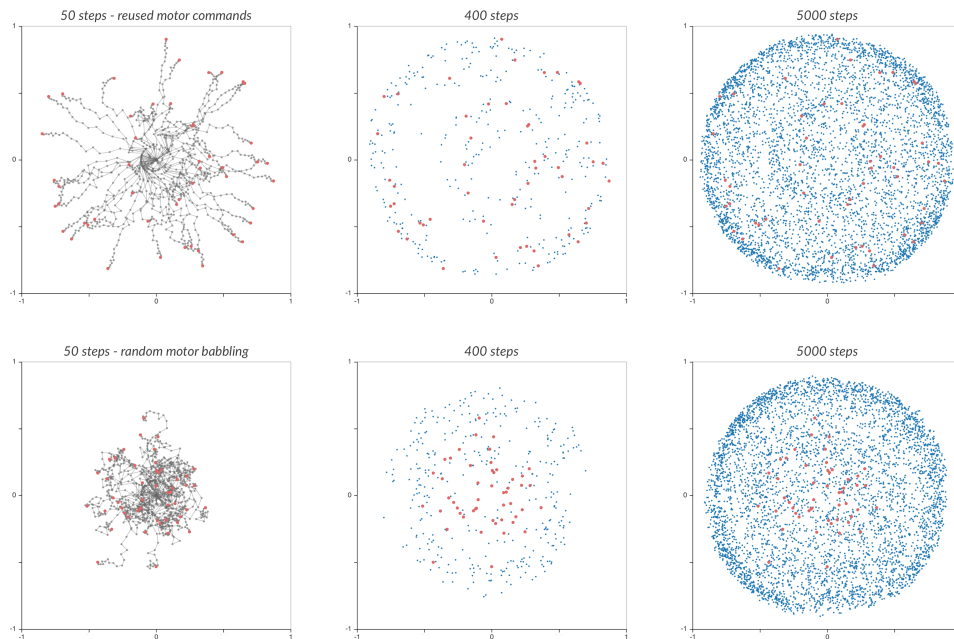
Figure 5.3: The benefits of the reuse exploration manifest mostly early in the exploration. Here, the top-most row shows an goal babbling exploration backed by reuse, while the bottom row shows a regular goal babbling exploration. In red, in the case of reuse, the effects produced by the reused motor commands, and in the case of regular random goal babbling, the effects produced during the 50-steps random motor babbling initial phase. [source code]
