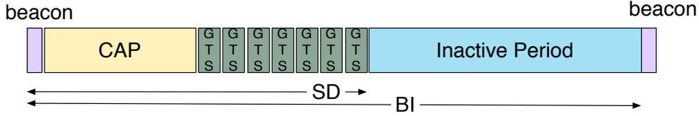
Figure 2.5: Superframe structure for IEEE 802.15.4 synchronous mode
