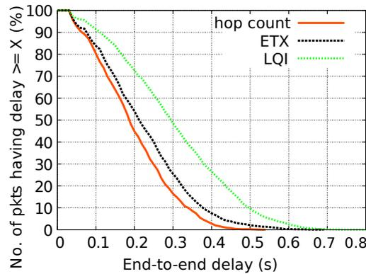
Figure 4.5: Complementary CDF of the end-to-end delay
