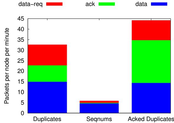
Figure 3.5: Overhead — 1 broadcast packet every 20s, CBOP algorithm
