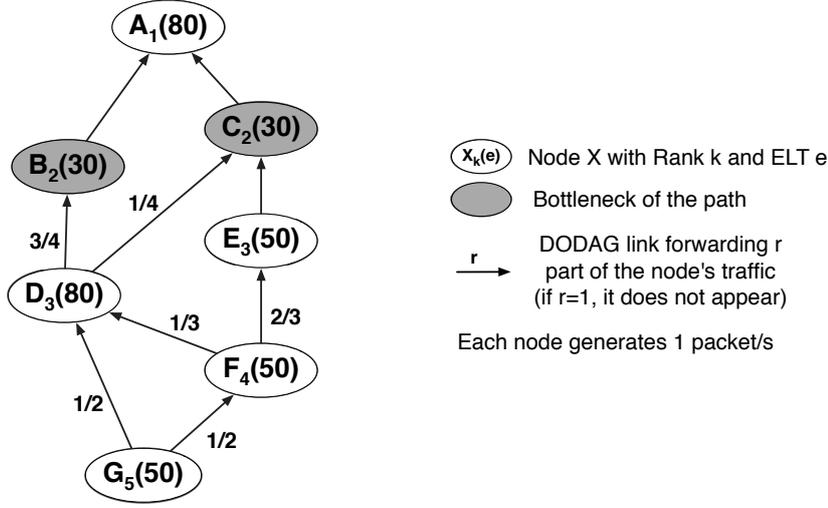
Figure 6.1: Path selection with ELT ( $\text{MinHopRankIncrease}=1$ )
