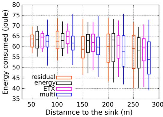
Figure 6.10: Energy consumption of nodes in function of their physical distance to the sink
