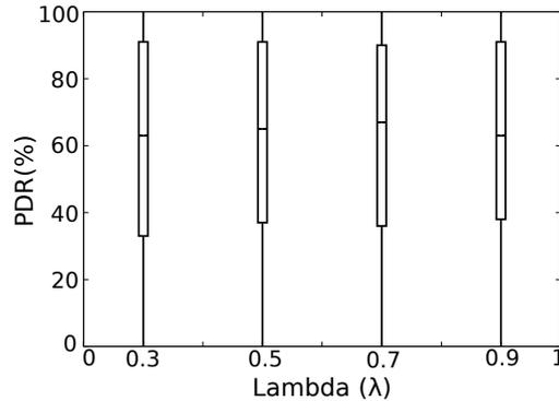
Figure 4.2:  $\lambda$  versus the packet delivery ratio, with ETX
