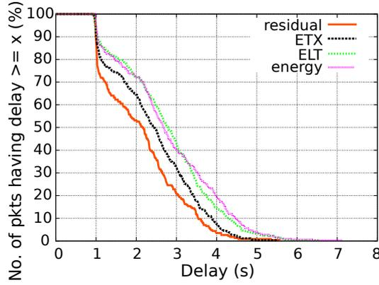
Figure 5.6: Complementary CDF of the end-to-end delay
