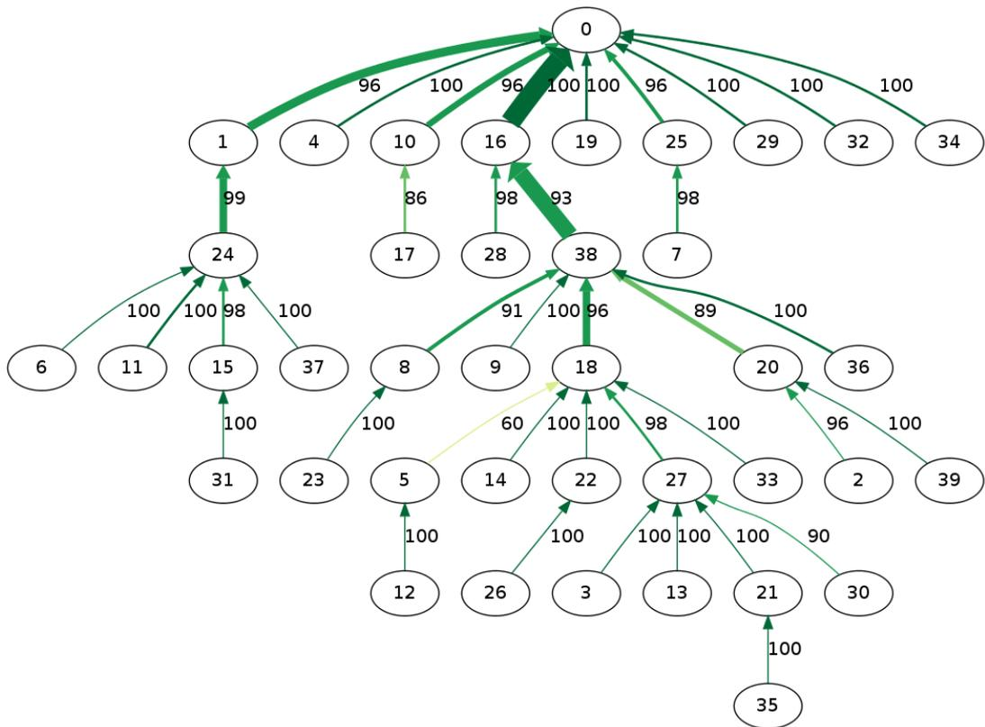
(b) Using ETX as a routing metric
