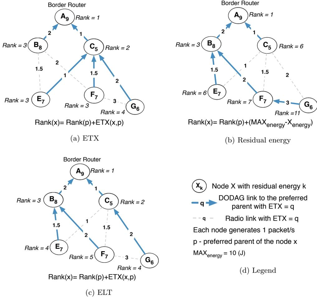
Figure 5.1: DODAG construction using different routing metrics
