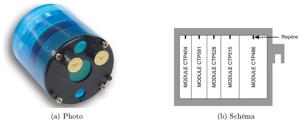
FIGURE 6.2 – fantôme Catphan<sup>®</sup> 600
