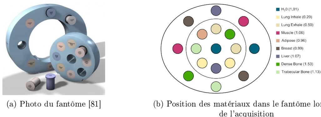
FIGURE 4.10 – Fantôme "Electron Density" de CIRS
