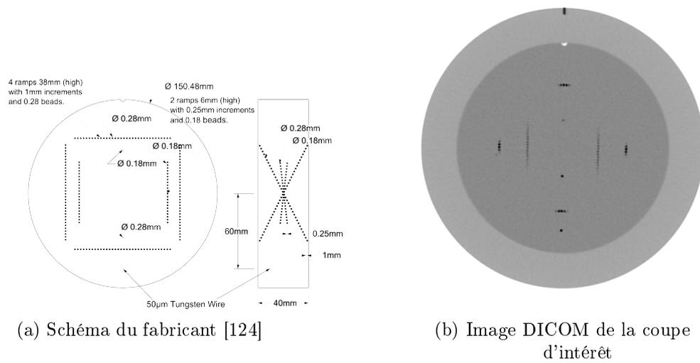
FIGURE 6.5 – Module CTP591 du fantôme Catphan<sup>®</sup>
