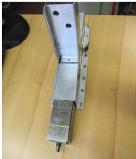
**Figure 5-4.** Stiffness block placed inside the horizontal beam
