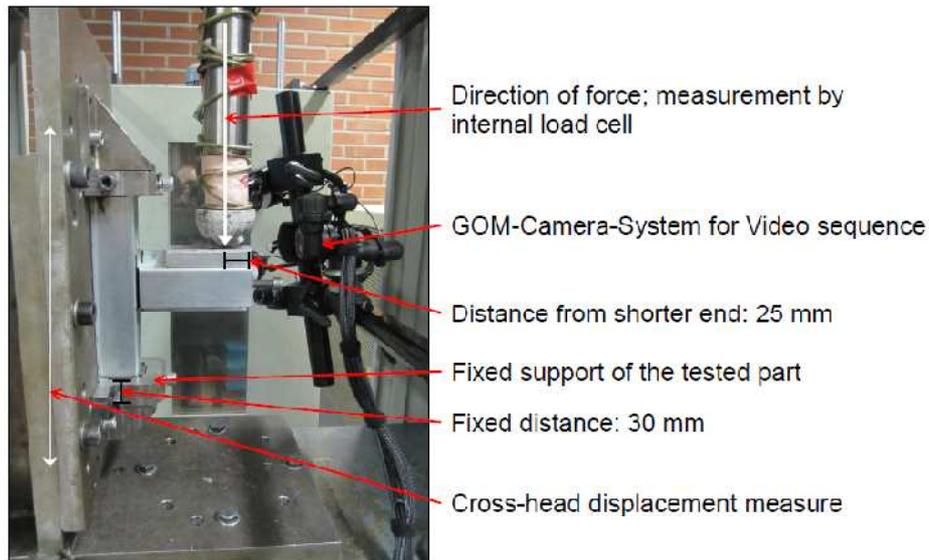
**Figure 5-5.** *T-joint test setup under longitudinal loading*
