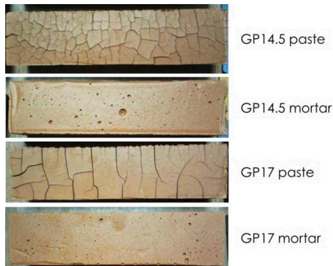
Figure 45. Surface cracking observed on 4x4x16 geopolymer samples for GP14.5 paste and mortar and GP17 paste and mortar.
