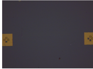
Figure 2.19: Cross alignment marks. In yellow the mark made by the contact deposition.
