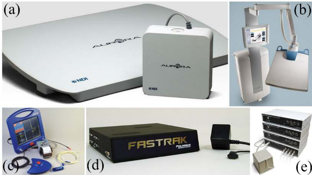
Figure 2.5: Commercial Electromagnetic trackers: (a) Northern Digital Inc Aurora® [NDI ], (b) Calypso EM tracker [Varian ], (c) Cortrack [Corpack-Medical ], (d) Fastrak by Polhemus [Polhemus ], (e) Ascension TrackSTAR and driveBAY [Ascension-tech ].
