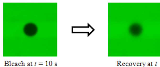
Figure 2.11: FRAP technique uses the high power of a laser to photobleach a defined region of the sample. The recovery of the fluorescence in this region indicates any kind of movement (diffusion or transport) of fluorescent molecules. The disc diameter, d , of the bleached region equals 115.17 \mu\text{m} .
