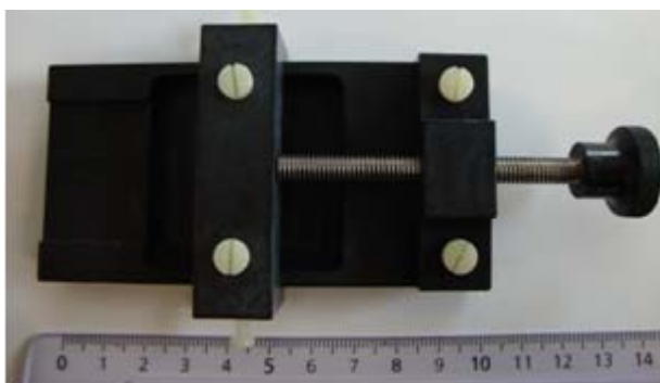
Figure 2.5: Stretching device used for the experiments where the modification of PDMS required extreme conditions as UVO activation or chemical contact.
