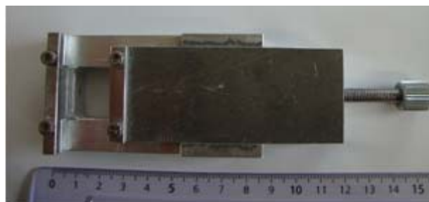
Figure 2.4: Medium stretching device use for the stretching of PDMS-hydrogel modified surfaces.
