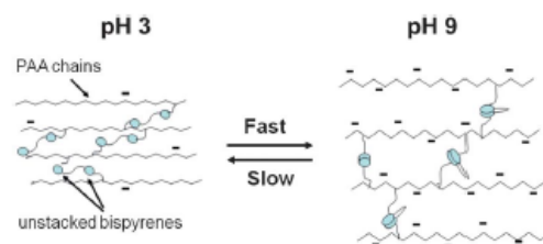
Scheme 4 Schematic representation of PAA-Alk/Az-bispyrene-Az films at pH 3 and 9. At pH 3, the PAA chains are less negatively charged and can get closer to each other whereas the amine functions of bispyrene spacers are protonated, leading to an opened form of the molecule. At pH 9, the bispyrene spacers adopt their unstacked conformations whereas the deprotonated carboxylic groups of PAA lead to electrostatic repulsion between the polymer chains.
