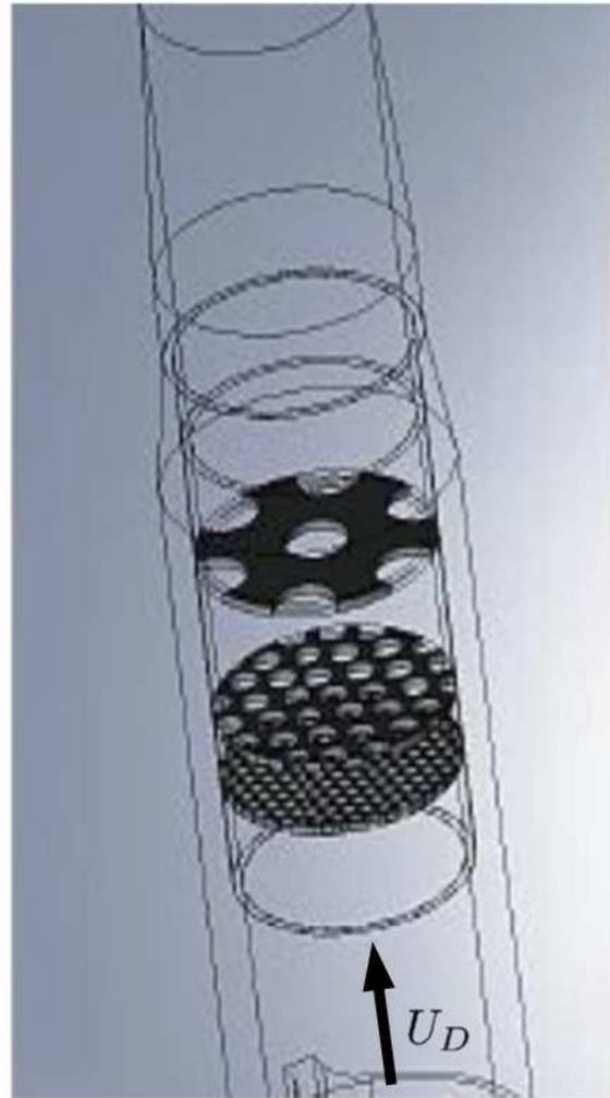
According to this relationship and the values reported in Table 1 we find  $d_{eq} \approx 2.5$  mm. The pressure drop coefficient  $K_j$  of the  $j$ -th perforated plate is defined as [17, 29]
