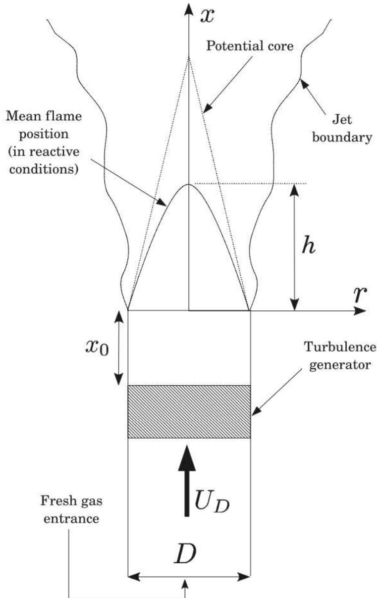
**Fig. 1** Schematic of the burner experimental set-up
