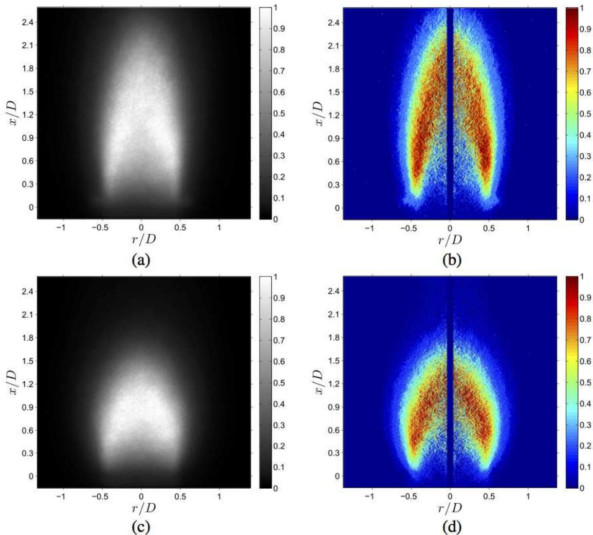
**Fig. 14** Averaged light emission collected for **a** single- and **c** multi-scale grids at  $P_{\text{int}} = 0.5$  MPa and the related Abel transform **b** and **d**, respectively. The colormaps represent the normalized light intensity
