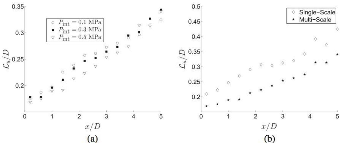
**Fig. 8** **a** Evolution of  $\mathcal{L}_u$  vs distance from the burner exit normalized by the burner diameter  $D$  (multi-scale grid). **b** Comparison of  $\mathcal{L}_u$  generated by single- and multi-scale grids ( $P_{\text{int}} = 0.5$  MPa)
