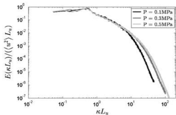
Fig. 7. Dimensionless 1D energy spectra.
