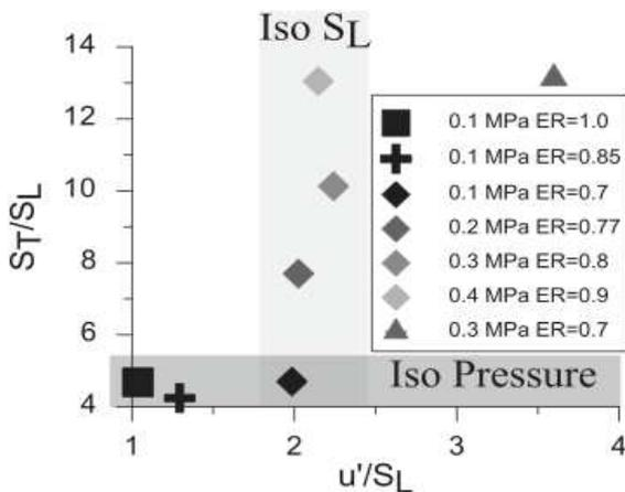
Fig. 4. Combustion intensity ( $S_T/S_L$ ) variations with  $u'/S_L$ .
