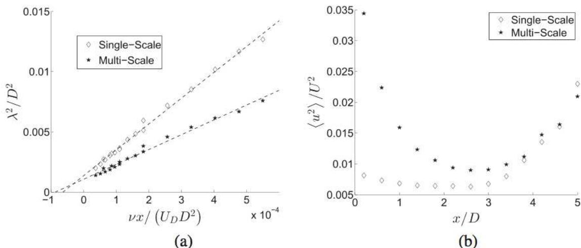
**Fig. 13** **a** Effect of internal pressure on the Taylor microscale. The dashed lines represent the best fits of Eq. (15) in the least square sense. **b** Streamwise evolution of the dimensionless normal Reynolds stress  $\langle u^2 \rangle$  along the jet axis ( $P_{\text{int}} = 0.5$  MPa)
