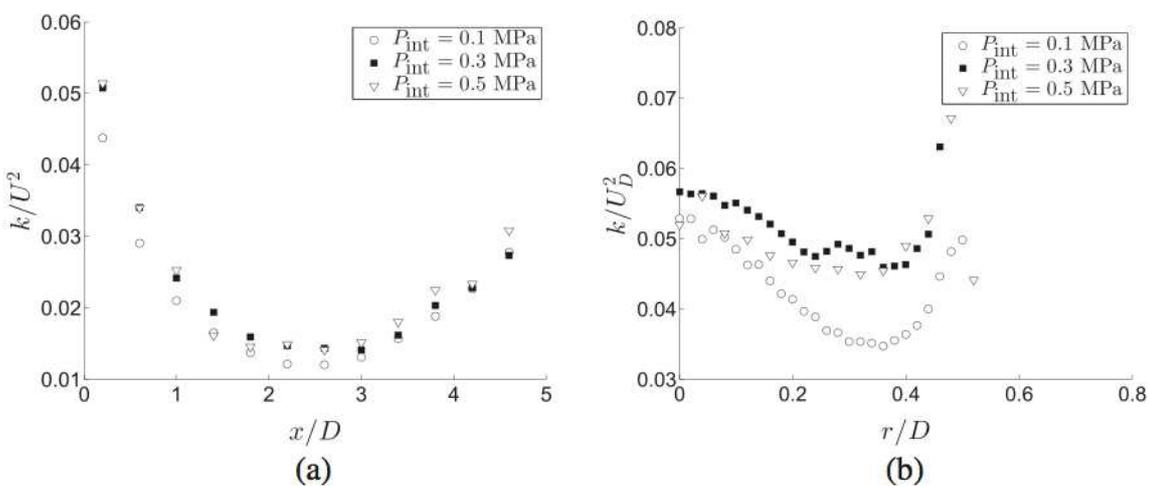
**Fig. 5** **a** Evolution of the turbulent kinetic energy along the burner axis (LDV measurements). **b** Radial profiles of the turbulent kinetic energy close to the burner exit ( $x/D = 0.2$ , LDV measurements)
