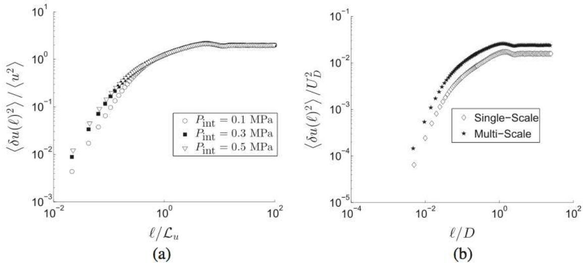
**Fig. 11** Evolution of the second-order structure function normalized by **a**  $D$  and  $U_D$  and **b** by  $\mathcal{L}_u$  and  $\langle u^2 \rangle$  ( $x/D = 1.8$ ,  $P_{\text{int}} = 0.5 \text{ MPa}$ )
