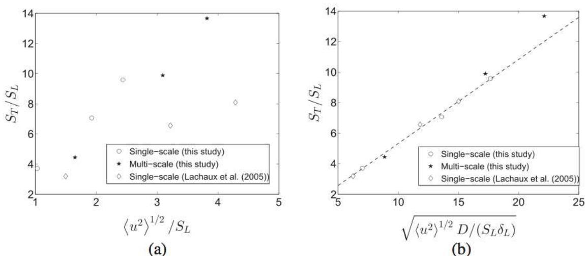
**Fig. 15** Variation of  $S_T/S_L$  vs **a**  $\langle u^2 \rangle^{1/2} / S_L$  and **b**  $\sqrt{\langle u^2 \rangle^{1/2} D / (S_L \delta_L)}$ . The dashed line represents the best linear fit in the least square sense of the data obtained for the single-scale grid
