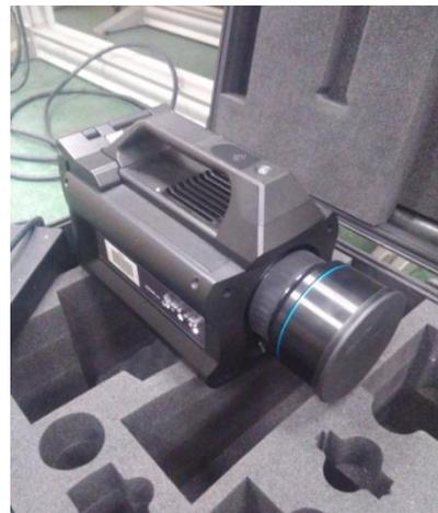
*Figure 2.15 - Caméra infrarouge FLIR X6540sc.*
