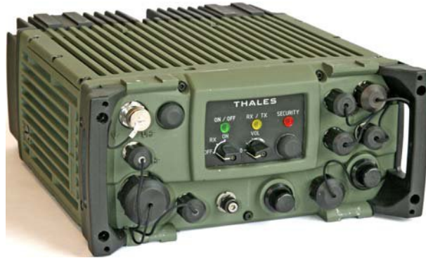
Figure 1.2: FlexNet. Vehicular wideband SDR platform sold by Thales Communications and Security.
