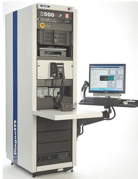
Figure 2.2: Automated RF test equipment ATE500 developed by DiagnoSYS
