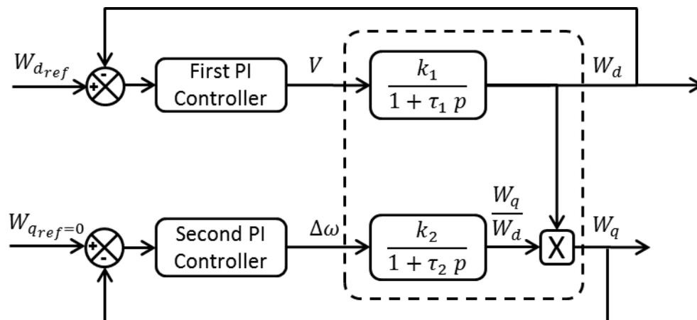
Figure 2-16: Control loops able to impose  $W$  and to operate the system at the resonance.
