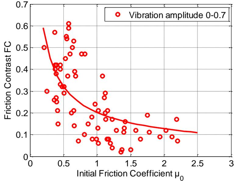
Figure 3.12: Friction contrast obtained from the experiment with a VA from 0 to 0.7  $\mu\text{m}$  as a function of the initial coefficient of friction  $\mu_0$  (VA = 0  $\mu\text{m}$ ) for both sliding velocities.
