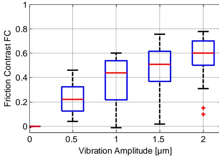
Figure 5-3: Friction contrast  $FC_{S-F}$  as a function of the VA from 0 to 2  $\mu\text{m}$ . The boxplot illustrates the difference between the six individuals participating in this tribological experiment (Ben Messaoud et al., 2015a).
