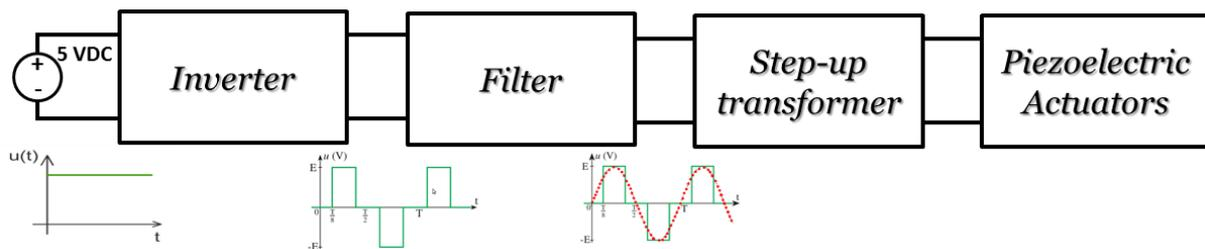
Figure 2-12: The power circuit to excite the piezoelectric ceramics by a controlled sinusoidal signal in amplitude and frequency.
