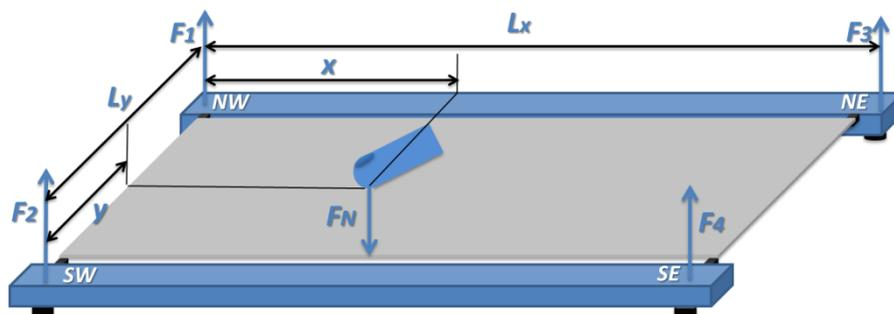
Figure 2-8: The designed configuration of the finger position estimation in  $x$  and  $y$  axes using four force sensors located in different locations: *NW (North West)*, *SW (South West)*, *NE (North East)* and *SE (South East)*.
