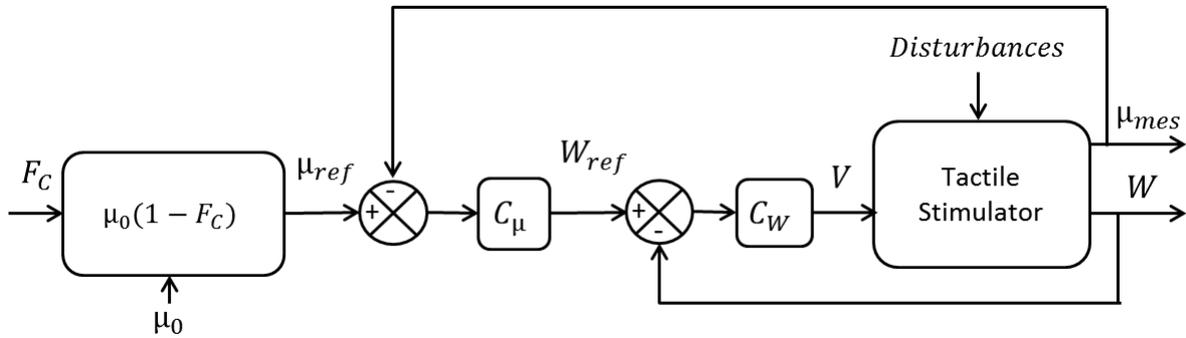
Figure 4-10: The operated control strategy to control the friction contrast between the fingers' users and the tactile plate. The reference  $FC$  is a function of the initial coefficient of friction  $\mu_0$  which is supposed to be constant.
