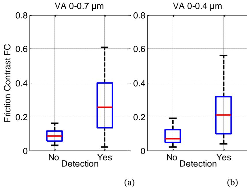
Figure 3.11: Boxplots of the friction contrast  $FC$  as a function of the tactile detection for the transition between 0–0.7  $\mu\text{m}$  (a) and 0–0.4  $\mu\text{m}$  (b) for both sliding velocities.
