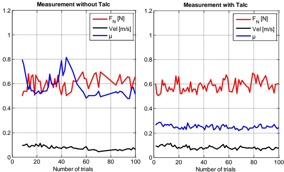
Figure 4-12: Result of the friction test with and without the talc powder on the finger. The normal force  $F_N$  and the finger velocity were in the same range for the two tests,  $0.5\text{ N} \leq F_N \leq 0.7\text{ N}$  and the velocity was about  $Vel\ 80\text{ mm/s}$ . The coefficient of friction  $\mu$  was variable without the Talc and almost constant even if reduced as expected when using the talc powder.
