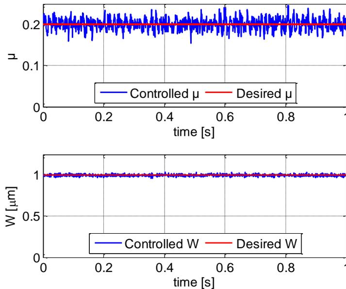
Figure 4-14: The controlled response of  $\mu$  and  $W$  for a constant desired reference.
