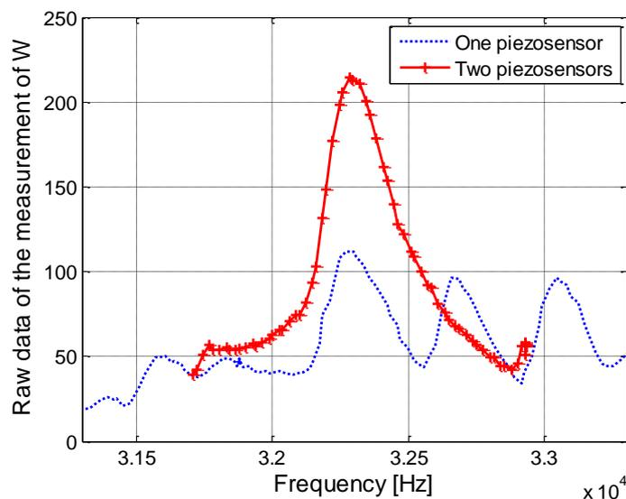
Figure 2-5: Comparison between using one or two piezo sensors when exciting the plate around resonance. The two-sensor approach emphasises the desired mode.
