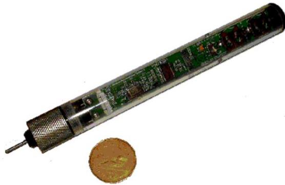
Figure 1-10: The WHaT prototype used to measure the contact force and the acceleration between the device and the real surface (Pai and Rizun, 2003).
