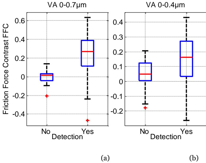
Figure 3.10: Boxplots of the friction force contrast  $FFC$  as a function of the tactile detection for the transition between 0–0.7  $\mu\text{m}$  (a) and 0–0.4  $\mu\text{m}$  (b) for both sliding velocities.
