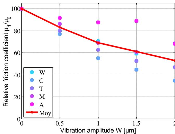
Figure 4-4: The ratio between the reduced friction  $\mu_1$  and the initial friction  $\mu_0$  in % depending on the vibration amplitude for five subjects plotted by colored points. The mean of measurements of all subjects is plotted by a continuous red curve.
