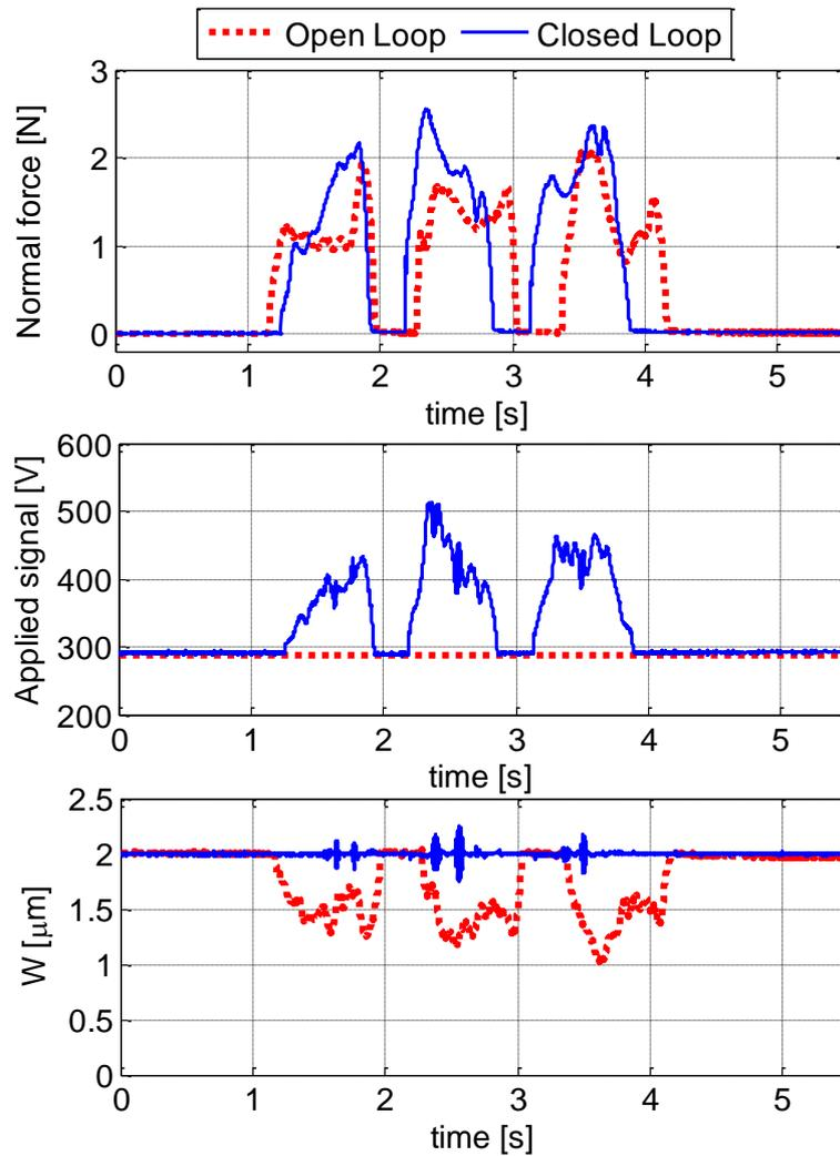
Figure 2-28: A comparison between the open and closed loop control when the finger is sliding on the plate excited at 2  $\mu\text{m}$  (peak to peak). As response to the normal force applied by the finger is between 0 and 2.5 N, it can be shown that the applied voltage signal to the piezoceramics reacts to ensure a stable level of vibration  $W$  with the closed loop control.
