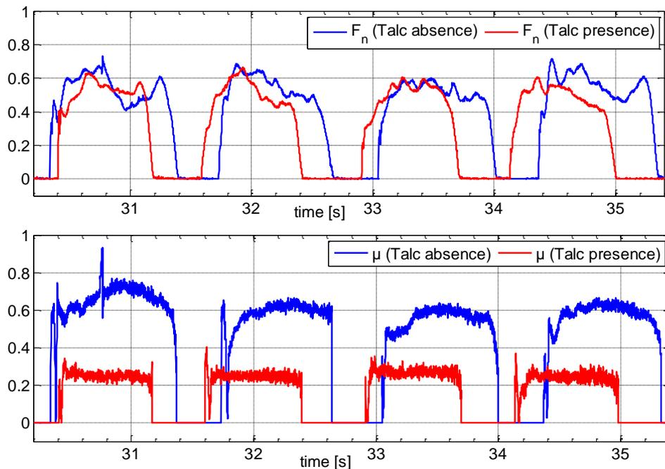
Figure 4-13: Evolution of the coefficient of friction  $\mu$  with and without talc powder, the normal forces are in the same range. Four cycles of friction are selected to show the difference between the two cases.
