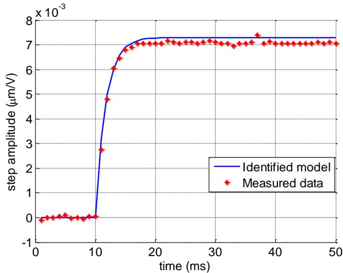
Figure 2-18: An example of one of the identified first order model, the voltage amplitude is 154 V peak to peak, giving  $K_1 = 7295$  (pm/V) and  $\tau_1 = 1.74$  ms.
