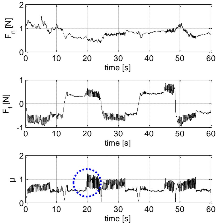
Figure 3.6: Normal force, friction force, and coefficient of friction of a subject sliding his or her finger on the tactile stimulator. Example of a female aged 46 years. The VA was  $0.7 \mu\text{m}$  and the sliding velocity was  $5 \text{ mm/s}$ .
