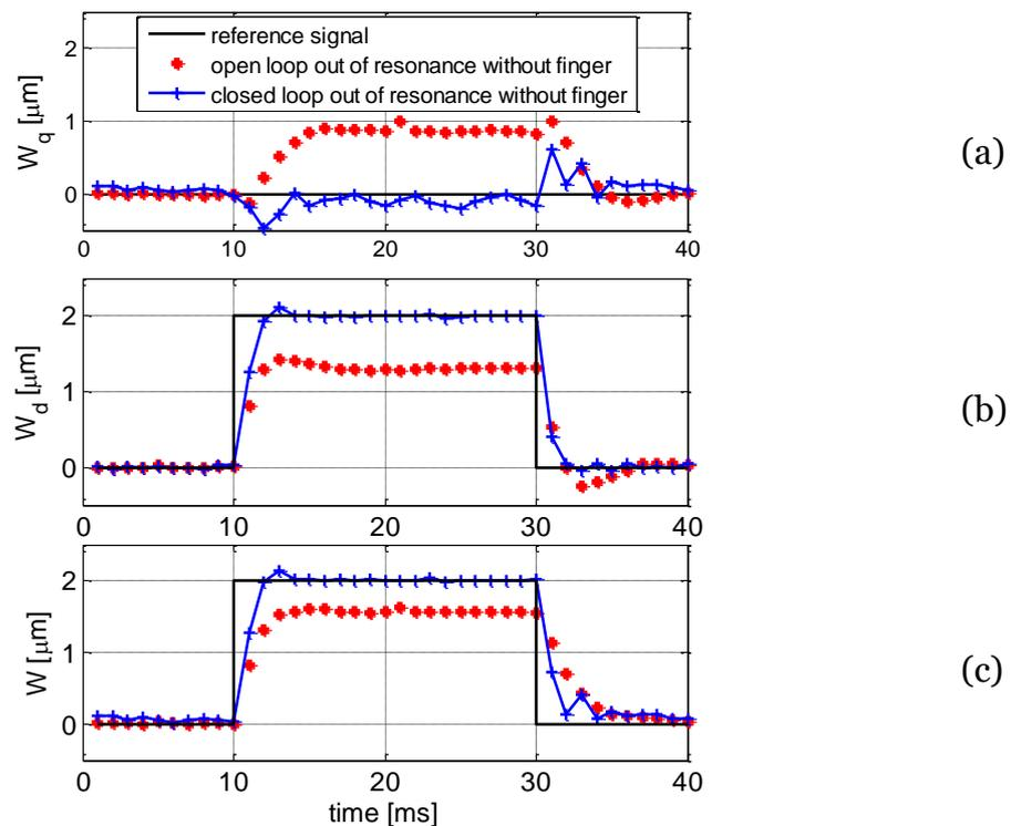
Figure 2-25 Response of the system in open and closed loop control when exciting the system as if it was at  $33^{\circ}\text{C}$  whereas the actual temperature is  $24^{\circ}\text{C}$  and without any finger force. Figures (a), (b) and (c) represent respectively the evolution of  $W_q$ ,  $W_d$  and  $W$  which is the module of  $W_d$  and  $W_q$ .
