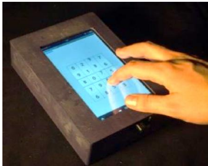
Figure 1-6: The TPad fire (Mullenbach et al., 2013)
