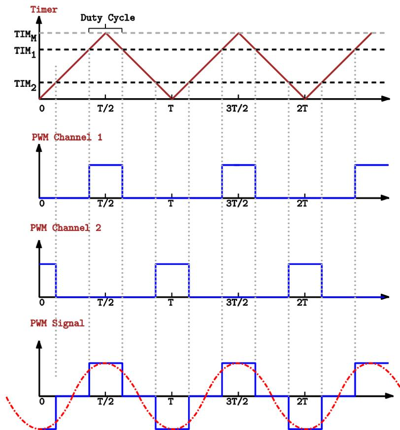
Figure A.1: The used method to create a three level PWM signal by the mean of two PWM signals with the same duty cycle and shifted by  $T/2$ . The sinusoidal voltage to be applied to the piezoceramics is filtered using a RL filter.
