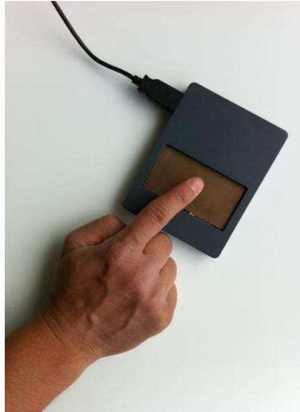
Figure 1-7: The optimized Stimtac version connected by a USB connection
