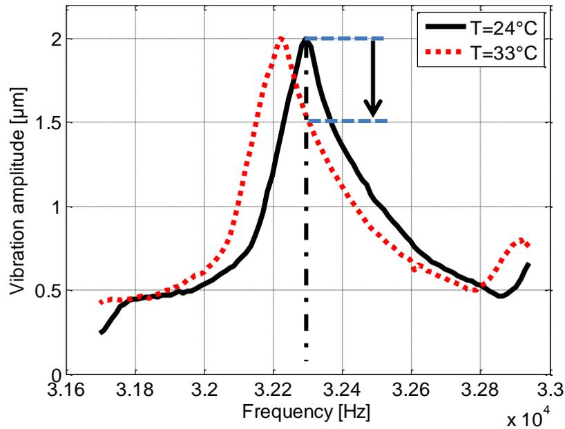
Figure 2-14: Frequency response around one mode for two stimulator's temperatures: 24°C (continuous, black line) and 33°C (dotted, red line).
