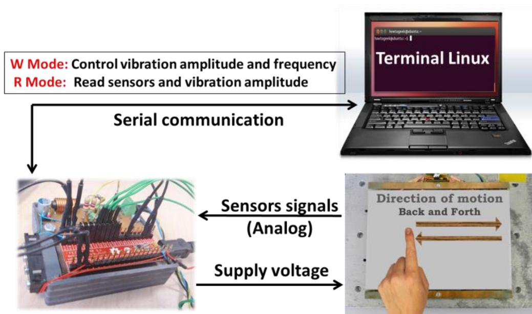
Figure 2-11: Operation principle of the tactile stimulator
