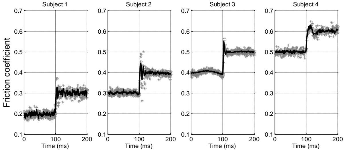
Figure 4-8: Closed loop control of the coefficient of friction as a function of time for the four subjects. The dotted curves illustrate at least four trials of touching the surface and the black continuous curve represents the average of all four measurements for each subject.
