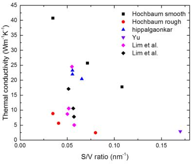
**Figure IV.4** Thermal conductivity of various Si nanowires at room temperature extracted from the literature [64,115–117] as a function of the S/V ratio.
