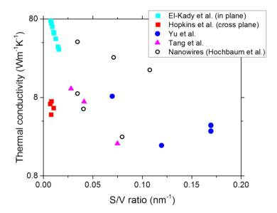
**Figure V.2** Thermal conductivity measurements extracted from the literature for 2D PnCs. Squares correspond to in-plane and cross-plane measurements done on similar structures [127,129]; circles correspond to different types of nanostructures with very small dimensions [64] and triangles are holes arranged in an hexagonal lattice [128]. Nanowires [115] are displayed for reference (open circles).
