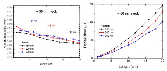
**Figure IV.19** Thermal properties of fishbone PnCs with a neck width about 50 nm at 4 K. (a) Thermal conductivity of fishbone structures with three different periods and (b) thermal decay times of these same structures.
