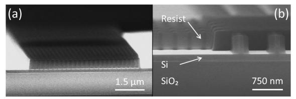
**Figure III.3** Samples after the second development step. (a) Cross section of a 2D PnC after the development of the resist. (b) Cross section of a fishbone structure after the development of the resist.
