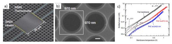
**Figure V.3** Engineered thermal conduction in periodic Si nitride membranes. a) SEM image of the phononic crystal with the heater and thermometer used for thermal conduction measurement. b) Close-up view of the PnC. The white square represents the zone covered by a unit cell and the scale bar has a length of 200 nm. c) Transmitted power for an unpatterned membrane as well as two PnCs designed to have lower coherent heat transport properties [41].
