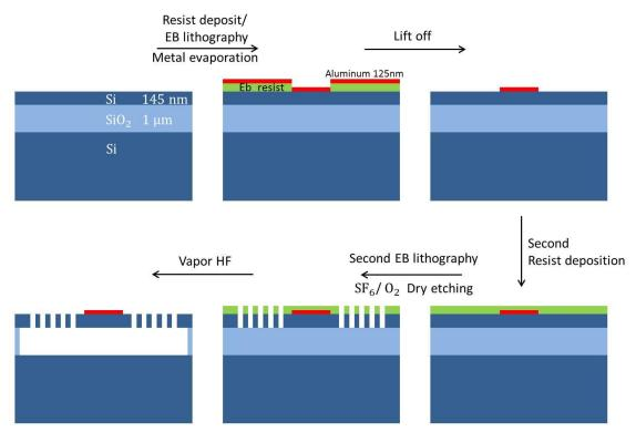
**Figure III.1** Flowchart of the fabrication process. The flowchart represents all the major steps in the fabrication process from a cross-sectional point of view. Included are the initial sample, the metal deposition, the lift-off, the second resist deposition, the plasma etching and, lastly, the buried oxide removal steps.
