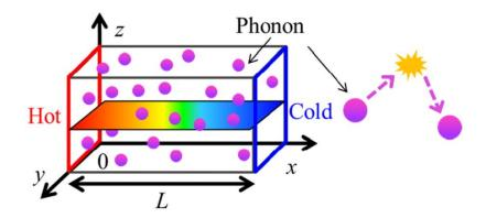
**Figure II.4** Schematic diagram of the Monte-Carlo simulation unit cell. The heat flux is determined by the boundary conditions. Scattering events are calculated within the simulation domain.
