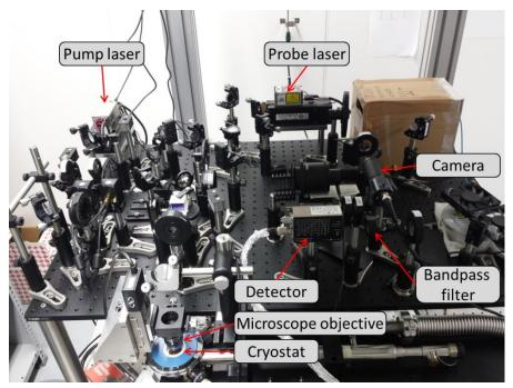
Figure III.11 Global view of the optical measurement system.
