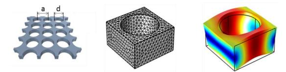
**Figure II.8** Schematic of a simulated periodic structure (left) with its unit cells demonstrating the mesh (center) and displacement fields (right) in one of the solutions. a represents the period and d the diameter of the holes.
