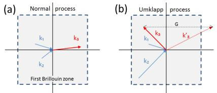
**Figure II.1** Schematic representation of (a) the Normal scattering process (N- Process) and (b) the Umklapp scattering process (U-Process) in the reciprocal space.
