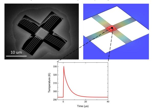
**Figure III.14** (left) SEM image of a nanowire nanostructure. (right) 3D model of the measured structure. All size parameters are faithfully taken from SEM images. The picture has been taken during the decay, when heat has started to spread across the structure. (lower) Time dependence of the temperature taken in the center of the metal pad.
