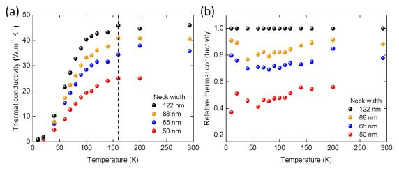
**Figure IV.16** Fishbone structures with varying neck width at temperatures ranging from 10 to 300 K. (a) Thermal conductivity for 4 sets of fishbone structures with period of 300 nm and  $W_{\parallel}$  of 140 nm and ( $W_{\perp}$ - neck width) = 388  $\pm 5$  nm, versus temperature. (b) Thermal conductivity of the same structures relative to that of the largest neck width.
