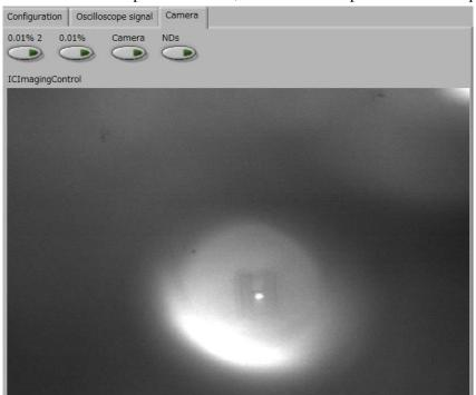
**Figure III.12** Optical microscope image of a sample mounted in the cryostat, with the laser beams hitting the central metal pad.
