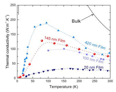
**Figure IV.3** Thermal conductivity of the bulk (black line) and the suspended thin film 145 nm in thickness (red) from 4 to 300 K. Other experimental points on 20 nm (down triangle), 100 nm (square) and 420 nm thick thin film (upper triangle) are extracted from the literature[105]. The dashed lines are B-splines and are displayed for clarity.
