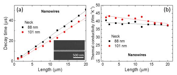
**Figure IV.8** Room temperature measurement of 2 nanowire sets with varying length. Points are experimental data while lines are linear fits. (a) Decay times as obtained from the optical measurement system. (Inset) SEM image of a single nanowire. (b) Effective thermal conductivity obtained from 3D FEM simulations.
