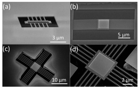
**Figure III.6** SEM images of completed structures of each type. (a) SEM image of a nanowire structure. (b) 2D PnC with a hexagonal lattice. (c) 1D fishbone structure and (d) close-up on the fishbone structure central part.
