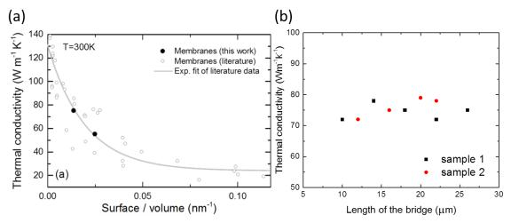
**Figure IV.2** (a) Measured thermal conductivity of suspended thin films of various thicknesses, from this work (80 nm and 145 nm thickness) and from the literature. The gray line is a fit of the literature data. (b) Length dependence of the thermal conductivity for a thickness of 145 nm.
