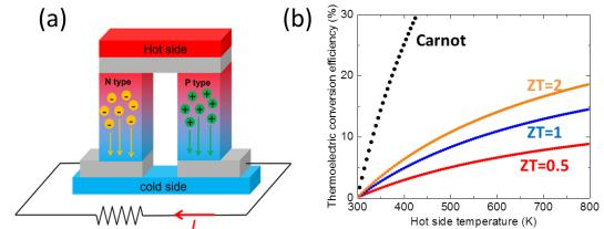
**Figure I.2** (a) Principle of a thermoelectric device and (b) Thermoelectric conversion efficiency as a function of the hot side temperature, when the cold side is fixed at 300 K, for different values of ZT.
