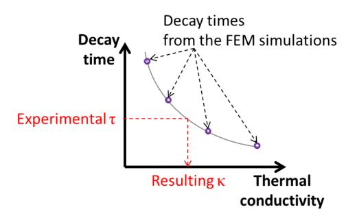
**Figure III.15** Thermal conductivity estimation process: Decay times are extracted from the FEM simulations and then linked by an exponential function. The decay time  $\tau$  obtained experimentally is plugged into this function, giving the corresponding thermal conductivity  $\kappa$  as output.
