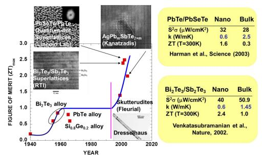
Figure I.4 History of the thermoelectric figure of merit [9].
