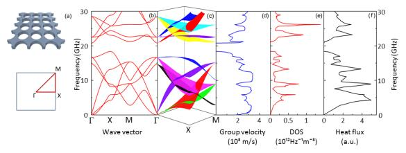
**Figure II.9** (a) Scheme of the simulated structure together with its first Brillouin zone and the high symmetry points  $\Gamma$  (0, 0), X ( $\pi/a$ , 0), and M ( $\pi/a$ ,  $\pi/a$ ). Phonon dispersion on the boundaries (b) and inside (c) of the irreducible triangle with a = 160 nm, r/a = 0.45, and h = 80 nm. Spectra of the average group velocity (d), density of states (e) and heat flux (f) [43].
