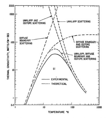
**Figure II.2** Comparison of the temperature-dependent thermal conductivity of Si between experiment and simulation [34].
