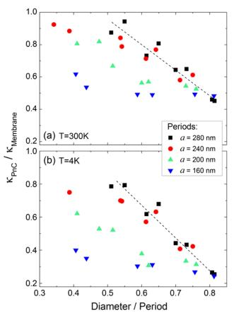
**Figure V.8** Thermal conductivity of the 2D PnCs relative to that of the unpatterned suspended thin film of same thickness at (a) room temperature and (b) 4 K for a variety of hole diameters. Colors represent different periods as indicated in the onset. Dashed line are linear fits of the data on structures with a = 280 nm.
