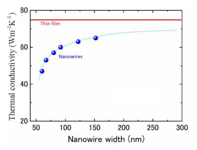
**Figure IV.6** Nanowire thermal conductivity for different widths at room temperature (blue) with a polynomial fit (blue dashed line) and the value of the thin film thermal conductivity (red).
