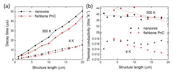
**Figure IV.12** Comparison between nanowires and fishbone structures of same width. (a) Decay times of both structures at room- and low-temperature and (b) corresponding thermal conductivities at the same temperatures.
