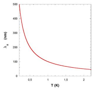
Figure II.6 Dominant wavelength as a function of temperature calculated from Eq. 2.24.
