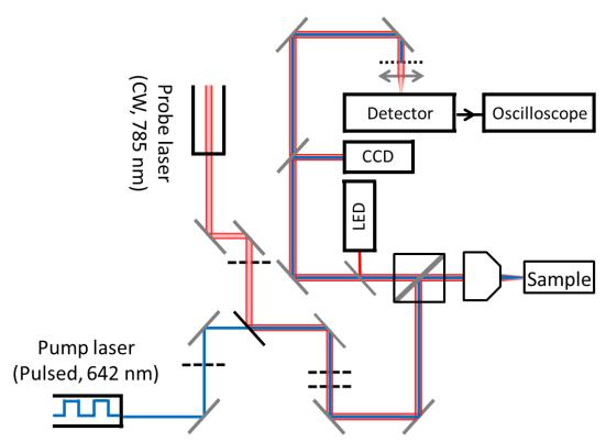
**Figure III.10** Schematics of the TDTR setup. Gray lines are mirrors. Black dashed lines are ND filters. The small dashes and the double-arrow in front of the detector are the band-pass filter and lens, respectively.
