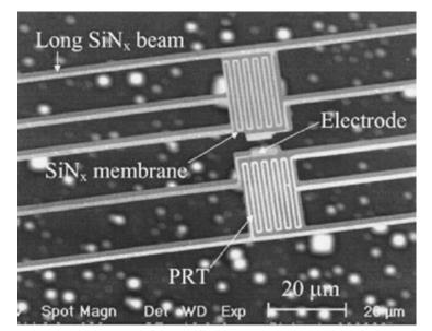
**Figure III.7** SEM image of an electrical measurement platform showing all the electrical wires [57]. The structure under study is placed between the 2 central electrodes. PRT stands for Platinum resistive heater, which can act both as a heater and a sensor.
