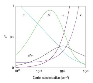
**Figure I.3** Evolution of the Seebeck coefficient  $\alpha$  (blue), the electrical conductivity  $\sigma$  (brown) and the thermal conductivity  $\kappa$  (violet), as well as the resulting power factor (black) and figure of merit (green) versus carrier concentration. The trends are extracted from the literature [5] and modelled for Bi<sub>2</sub>Te<sub>3</sub>.
