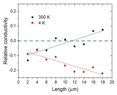
**Figure IV.20** Relative thermal conductivities of two sets of fishbone PnCs with a period of 150 and 300 nm. Measurements were performed both at room (black) and low temperature (red).
