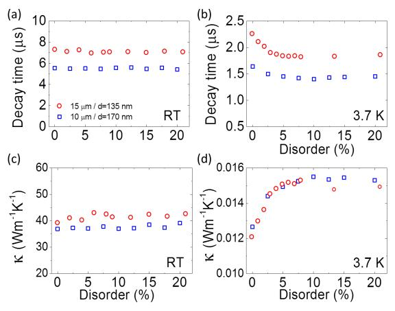
**Figure V.12** Decay times and thermal conductivity of the thermocrystals (a) Measured decay times for two different thermocrystals with hole diameters d = 135 nm (red) and d = 170 nm (blue) at room temperature. 10 and 15 µm represent the respective length of the thermocrystals as described in the fabrication section. (b) Decay times for the same structures at 3.7 K. (c) Corresponding effective thermal conductivities for the same set of structures at RT and (d) at 3.7K.
