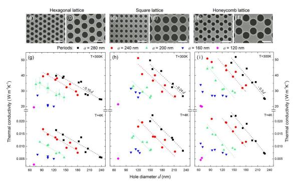
**Figure V.7** Thermal conductivity of various 2D PnCs. (a-f) SEM images of 2D PnCs with various arrangements of holes, such as hexagonal (a,b), square (c,d) and honeycomb (e,f) lattice types. Their respective thermal conductivities are plotted in panels g-I at room temperature (upper) and 4 K (lower) for periods of 120 nm (pink), 160 nm (blue), 200 nm (green), 240 nm (red) and 280 nm (black). Dashed lines are linear fits of the results with a fixed inclination per lattice type.
