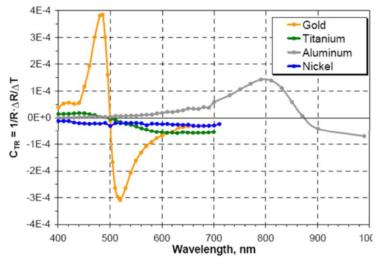
Figure III.8 Spectra of thermoreflectance coefficients for different metals [75].
