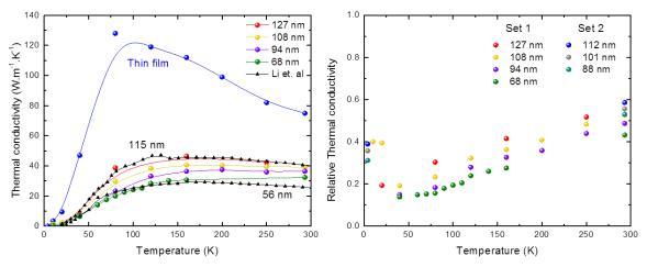
**Figure IV.7** (a) Temperature dependence of the thermal conductivity for the unpatterned thin film and nanowires of different widths between 10 and 300 K. (b) Calculated relative thermal conductivities of the nanowires as compared to the thin film. The missing values of the thin film thermal conductivities have been interpolated.
