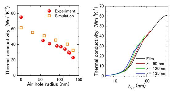
**Figure V.5** (a) Thermal conductivity of 2D PnCs with holes of various sizes arranged in a periodic square lattice of period 300 nm. (b) Accumulated thermal conductivity for similar structures calculated by MC simulations. The accumulated thermal conductivity is plotted as a function of the MFPs of phonons [130].
