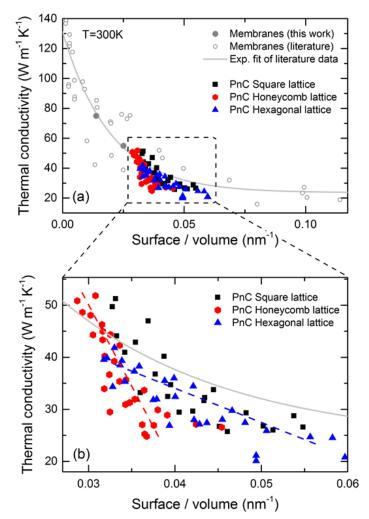
**Figure V.9** Thermal conductivity of 2D PnCs plotted as function of their S/V ratio at room temperature. The three different lattice types are represented by red circles for the honeycomb, blue triangles for the hexagonal and black squares for the square lattice type. In grey are plotted various unpatterned thin films from the literature, as well as our own work.
