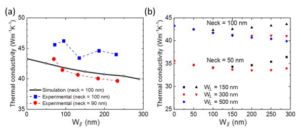
**Figure IV.14** Dependence of the thermal conductivity in fishbone structures. (a) Experimental (blue and red) measurement versus MC simulations (black). (b) MC simulations at room temperature for structures of period 300 nm as a function of the different geometrical parameters.
