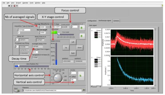
**Figure III.13** Main screen of the Labview program during measurement. All the commands are on the left. In the right part are displayed all the relevant curves: the base curve as output by the oscilloscope (red), the box-averaged curve (white), the decay of the box-averaged curve (blue) and the exponential decay fit (green line) superposed on the blue decay curve.
