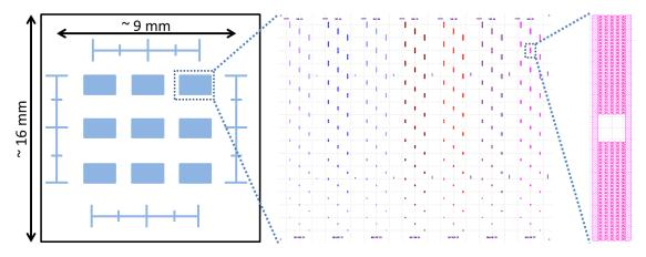
**Figure III.2** Global design of a chip with (a) the complete chip as processed, (b) the global positioning of the structures in a sub-chip and (c) a close-up view on the pattern file of a fishbone structure as is used for EB lithography.
