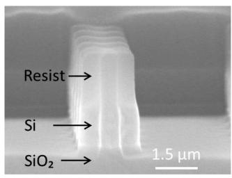
**Figure III.4** Cross-sectional SEM image of a fishbone structure after the ICP RIE step. The three visible layers from top to bottom correspond to the resist, the Si layer and the  $SiO_2$  box respectively.
