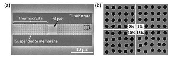
**Figure V.11** Fabricated structures and thermal conductivity measurement method for microstructures. (a) SEM image of a fabricated suspended Si thin film with holes arranged in a square lattice. (b) Close-up view of phononic nanostructures with different amount of disorders of 0, 5, 10, and 15%. The scale bar is 300 nm.
