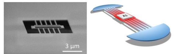
**Figure IV.5** (a) SEM image of a nanowire nanostructure. (b) Schematic of the suspended nanowires structure with the Al pad heater in its center. The color gradient represents the temperature during the thermal dissipation process. The temperature in the square Si island under the Al pad is considered uniform.
