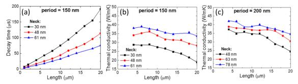
**Figure IV.18** Length dependence of the thermal properties of fishbone nanostructures.  $W_{\parallel}$  is equal to half the period while  $W_{\perp}$  is 455 and 470 nm for the structures of period 150 and 200 n respectively. (a) Decay times for 3 sets of structures with period 150 nm and varying neck and length. (b) Corresponding thermal conductivities for the same structures and (c) similar structures with period 200 nm.
