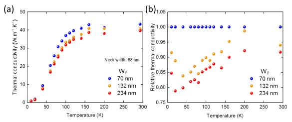
**Figure IV.17** Fishbone structures with varying  $W_{\parallel}$  at temperatures ranging from 10 to 300 K. The period is 300 nm and  $W_{\perp} = 474 \pm 4$  nm. (a) Thermal conductivity for 3 sets of fishbone structures versus temperature. (b) Thermal conductivity of the same structures relative to that of the smallest  $W_{\parallel}$ .
