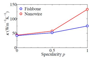
**Figure IV.13** Effect of the specularity parameter p on the thermal conductivity of rectangular cross-section nanowires (red) as well as fishbone PnCs (blue) calculated by MC simulations at room temperature. The period is 300 nm, the neck width 100 nm for both the nanowires and the fishbone structures.  $W_{\parallel} = 100$  nm and  $W_{\perp} = 300$  nm.
