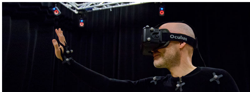
FIGURE 2.11 A tracking system that combines multiple infrared VICON cameras (in red) in order to track reflective marker patterns. By increasing the number of cameras used, the tracking zone (range) can be enlarged. Here, for a VR application, the system is used in order to track the user's body parts such as his hands and his head.
