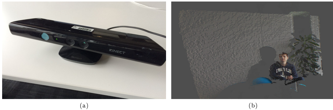
FIGURE 2.12 (a) The Microsoft ® Kinect ™ is an example of depth sensor that uses a structured light approach. (b) The point cloud provided by this sensor crosses the depth image with the RGB one.
