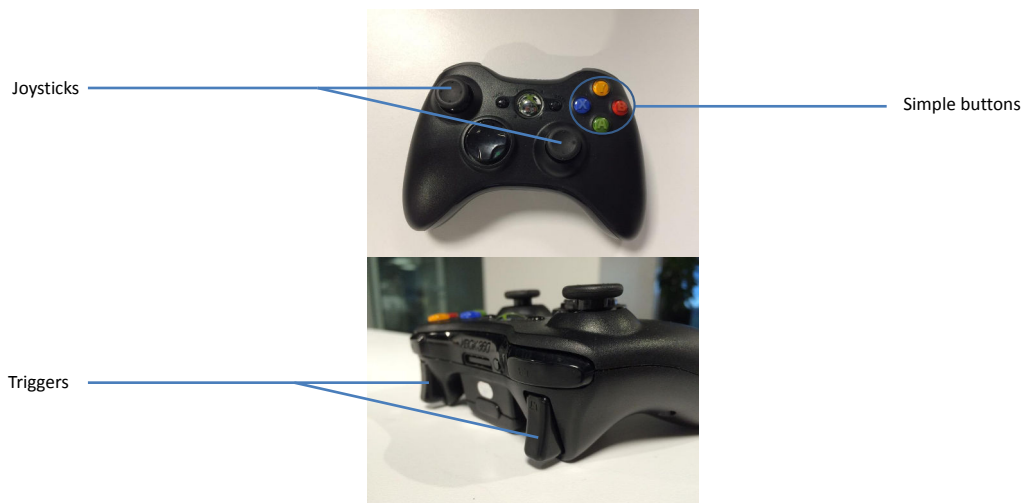
FIGURE 2.10 The Xbox360™ gamepad is a classic game controller composed of joysticks, triggers and simple buttons. This kind of device is commonly used for playing video games.
