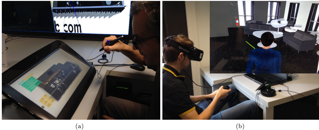
FIGURE 5.3 The collaborative extension of the furniture planning application (a) The customer is immersed with a first person view in the shared virtual world with a HMD and interacts with a Razer Hydra. (b) The guide has a 3/4 top view of the scene and uses the zSpace interactive system.
