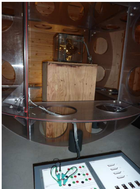
Figure 12 : Cross talk setup. Cassini sensor located within the new Helmholtz tri-axis coils and the rack GSE2 is located in the grounded mumetal box (not shown).
