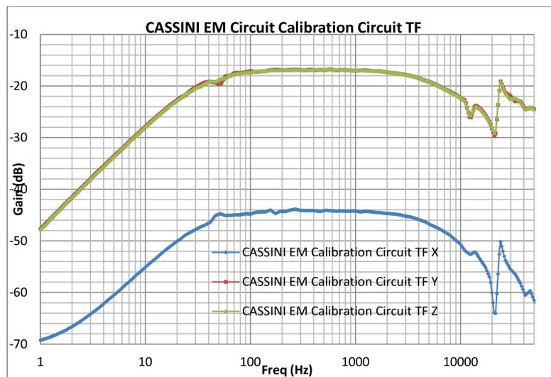
**Figure 7:** Cassini EM Calibration circuit transfer function (in Gain dB/V).
