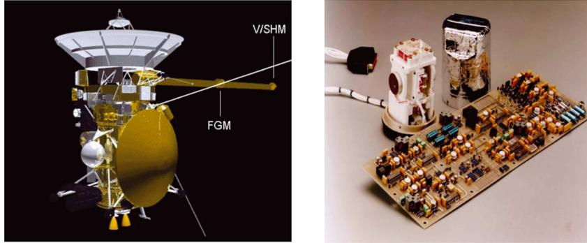
**Figure 4.3:** Left: The location of the magnetometer hardware on the spacecraft is shown halfway the "mag boom". Right: Electronics photograph of the FGM (with cover off) and electronics board. Adapted from Dougherty *et al.* [2002].
