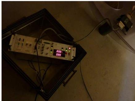
**Figure 2 :** Rack GSE2 (+12/-12V power supply) connected to Cassini EM PA and located to the mumetal box in order to reduce the 50Hz tone produced by the power supply. The mumetal box is grounded to the rack ground. The Y axis (red coaxial cable) is connected to the spectrum analyzer.
