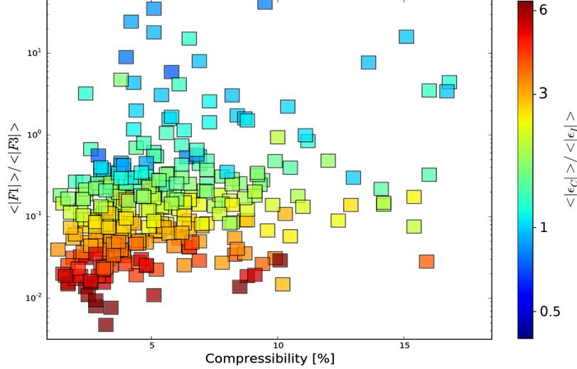
**Figure 5.26:** 2D plot of  $\langle |\mathcal{F}_1| \rangle / \langle |\mathcal{F}_3| \rangle$  as a function of the compressibility and the ratio  $\langle |\varepsilon_C| \rangle / \langle |\varepsilon_I| \rangle > 1$ .
