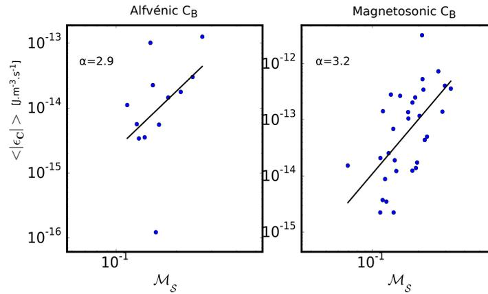
**Figure 6.6:** Compressible energy cascade rate as a function of the turbulent Mach number for the Alfvénic and the magnetosonic like events. The black line is a least square fit of the measurements with  $\alpha$  the corresponding fitting index.
