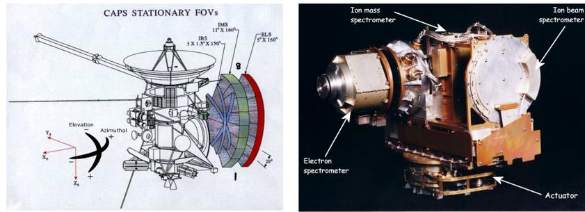
**Figure 4.6:** Left: Location of the CAPS sensors on Cassini spacecraft. Right: CAPS instrument with its three sensors (ELS, IMS, & IBS) and the actuator motor platform. Adapted from *Young et al.* [2004].
