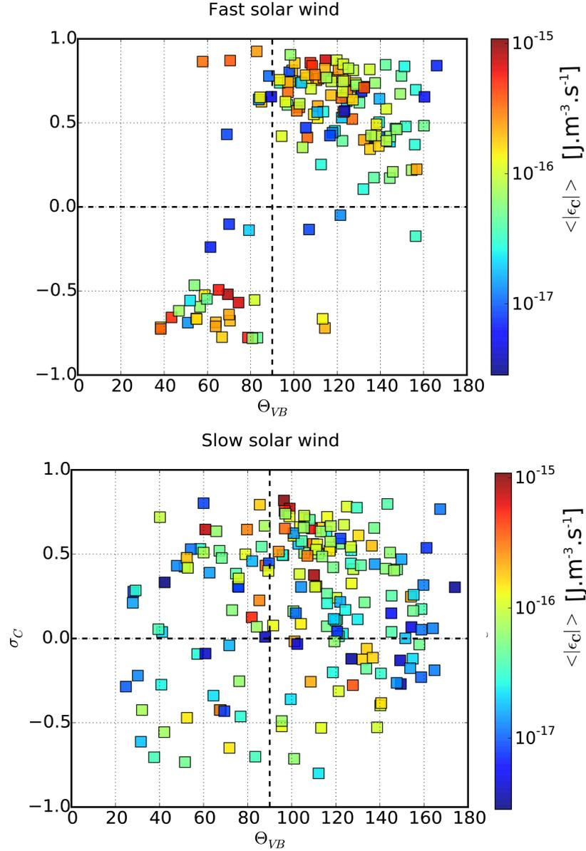
**Figure 5.21:** Cross-helicity ( $\sigma_c$ ) plotted as a function of the propagation angle  $\Theta_{\mathbf{VB}}$  and  $\langle |\epsilon_c| \rangle$  in the fast wind (Top) and the slow wind (Bottom). For an outward propagation,  $\sigma_c \sim +1$  and is anti-parallel to  $\mathbf{B}$ . Whereas for an inward propagation  $\sigma_c \sim -1$  and is parallel to  $\mathbf{B}$ .
