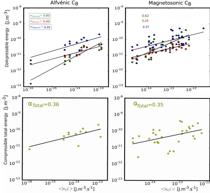
**Figure 6.8:** First Panel: the magnetic (blue), kinetic (red) and internal (green) energies of the compressible fluctuations in the terrestrial magnetosheath. Second Panel: the total compressible energy, plotted as a function of the compressible energy cascade rate  $\langle |\varepsilon_C| \rangle$ . The black lines are the least-square-fits with  $\alpha$  the corresponding fit coefficient.  $\delta E \sim \varepsilon_C^\alpha \rightarrow \varepsilon_C \equiv \delta E^{1/\alpha}$ .
