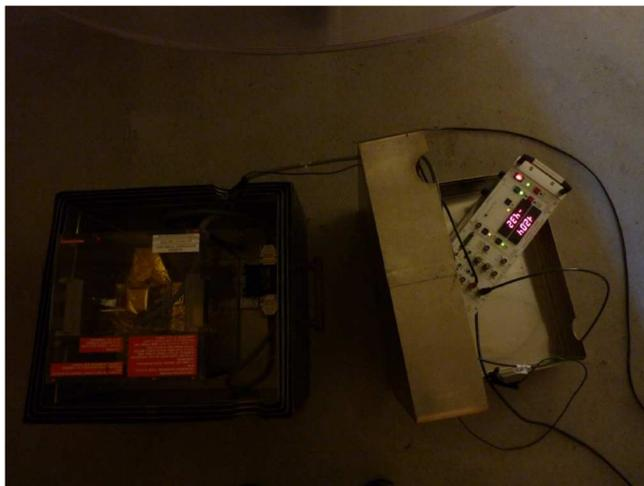
**Figure 9 :** Cassini EM sensor and PA inside the mumetal box for output noise measurement of the Y channel. The rack GSE2 has been covered with mumetal tops in order to reduce the 50 Hz tone.
