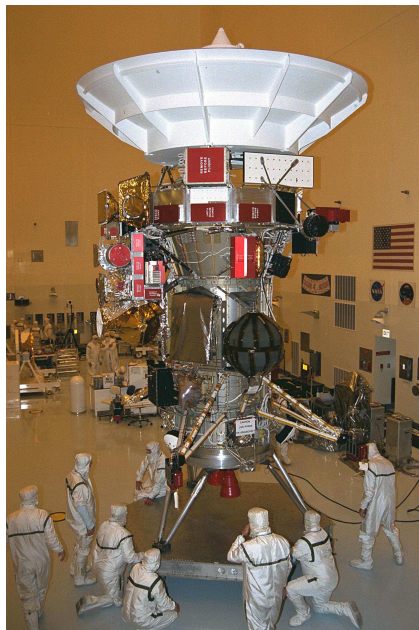
Figure 4.2: The Cassini-Huygens spacecraft assembly in Kennedy Space Center's. ©NASA Kennedy Space Center.
