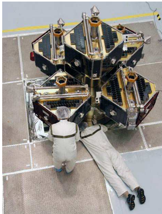
Figure 5.2: Top view of the five THEMIS spacecraft in their "wedding cake" configuration before spin-balance testing. ©NASA/George Shelton.
