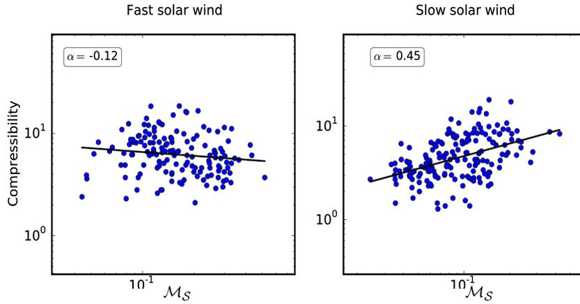
**Figure 5.14:** The compressibility  $(\sqrt{(\langle \rho^2 \rangle - \langle \rho \rangle^2)} / \langle \rho \rangle)$  as a function of the turbulent Mach number in the fast and the slow wind. The black line represents a least square fit of the data.  $\alpha$  is the corresponding correlation coefficient.
