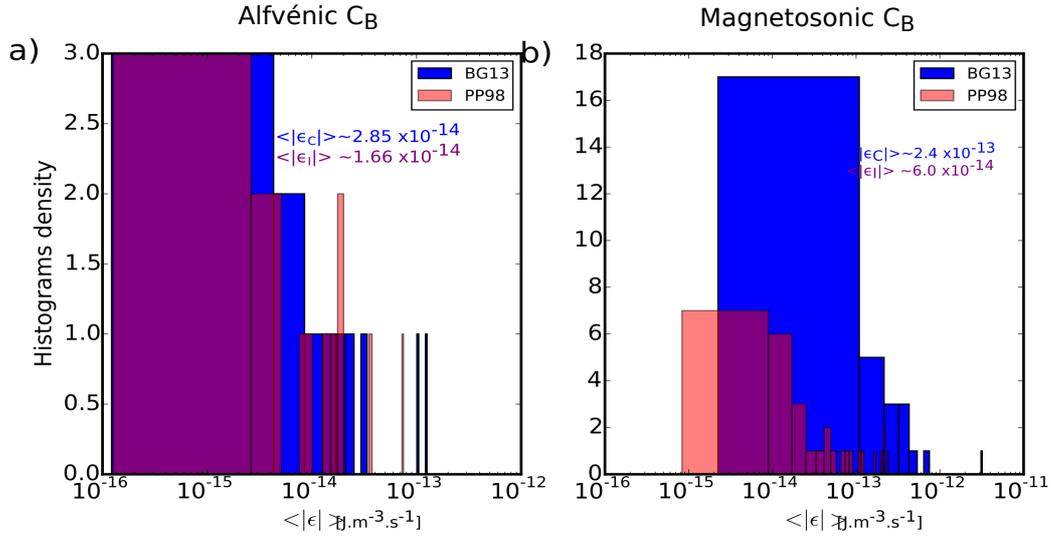
**Figure 6.4:** Histograms of the averaged values of the compressible energy cascade rate computed using BG13 (blue) compared with the incompressible one calculated using PP98 (red), for two groups of events: (a) showing and Alfvénic-like  $C_B$  and (b) a magnetosonic-like  $C_B$ .
