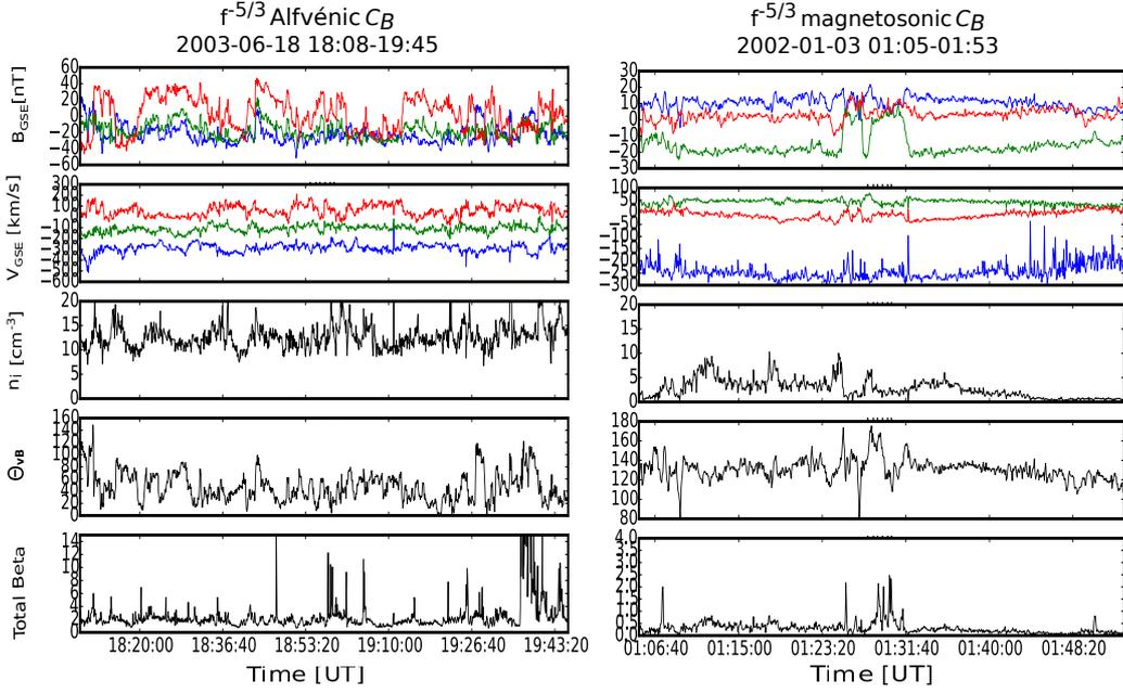
**Figure 6.2:** Magnetosheath events for which the inertial range is characterized by (left) an Alfvénic type of the magnetic compressibility and (right) a magnetosonic like one. From top to bottom: magnetic field vector, velocity vector, ion density, propagation angle  $\Theta_{\mathbf{vB}}$ , and the total plasma beta.
