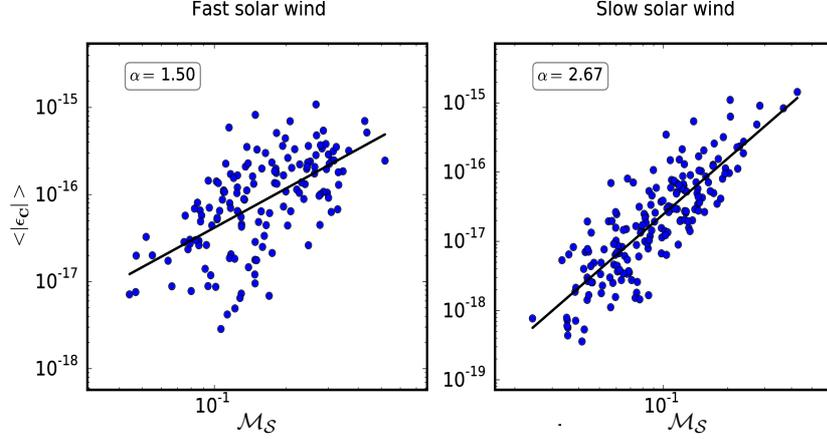
**Figure 5.13:** The absolute averaged energy transfer rate as a function of the turbulent Mach number in the fast and the slow wind. The black line represents a least square fit of the data in the log space.  $\alpha$  is the corresponding correlation coefficient.
