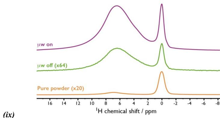
**Figure 2.**  $^1\text{H}$  Hahn-echo MAS NMR spectra of C-HAp, recorded at  $\sim 100$  K and 9.4 T. The pure powder (bottom, orange, MAS rate = 8.5 kHz) and the impregnated sample with (top, purple) and without (middle, green) microwave irradiation suitable for DNP (both recorded using a MAS rate of  $\sim 14$  kHz) are shown and scaled according to the numbers in parentheses.
