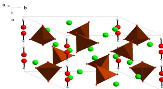
**Figure 1. Representation of the unit cell of hexagonal HAP,  $\text{Ca}_{10}(\text{PO}_4)_6(\text{OH})_2$ . Columns of  $\text{OH}^-$  (A-sites) are represented vertically (*c*-axis) (Ca in green, O in red, H in white,  $\text{PO}_4$  tetrahedra in brown). ICSD-26204: Hollysprings hydroxyapatite, showing the orientational disorder along the OH columns.**
