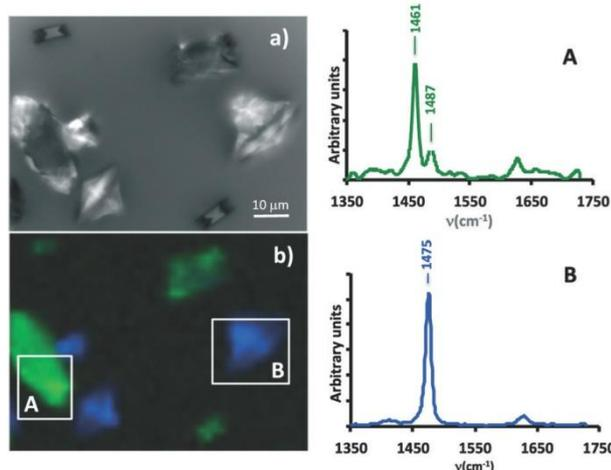
Fig. 3 a) Optical image of a portion of the microchannel, and b) corresponding Raman mapping for two spectral regions, 1452–1468  $\text{cm}^{-1}$  in green and 1470–1480  $\text{cm}^{-1}$  in blue. The Raman spectra A and B correspond to the A and B zones indicated in b).
