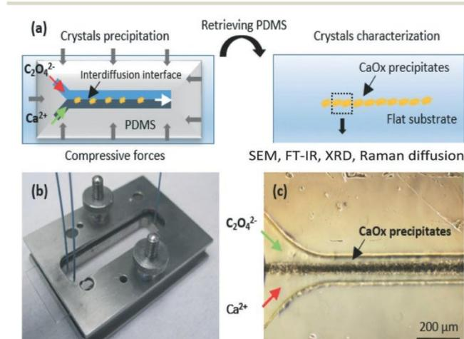
**Fig. 1** a) Principle of the dismantlable two-phase laminar flow microfluidic device used for the synthesis and characterization of precipitated CaOx crystals. b) Image of the microfluidic device assembled within the compressive metallic holder. c) Optical micrograph showing the “conic shape” precipitation of CaOx crystals at the dynamic interface in the zone of molecular interdiffusion.
