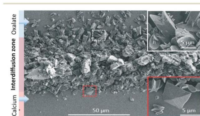
**Fig. 2** SEM image of precipitated crystals obtained in the microfluidic device from oxalate and calcium solutions at the dynamic interface. The white inset shows a zoom of the upper part of the precipitate containing twinned crystals. The red inset shows a zoom of the lower part of the precipitate containing mixed twinned and tapered bipyramid crystals.
