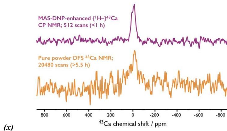
**Figure 3.**  $^{43}\text{Ca}$  MAS NMR spectra of C-HAp, recorded at  $\sim 100$  K, 9.4 T, and using a MAS rate of 8.5 kHz. Direct CT excitation of  $^{43}\text{Ca}$  after DFS of the pure powder (bottom, orange) is compared to the DNP-enhanced  $\{^1\text{H}\}\text{-}^{43}\text{Ca}$  CP experiment (top, purple), recorded using a CP contact time of 5 ms. Note that the time required to obtain much greater S/N with the DNP-enhanced experiment was  $< 1/5$  compared to the conventional method.
