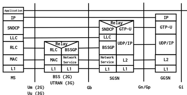
Figure 1.4 : Encapsulation GTP [3]
