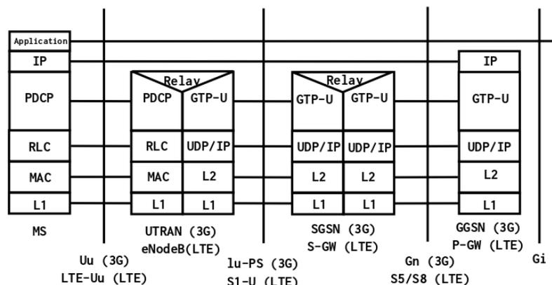
Figure 1.5 : Encapsulation GTPv2 [2].
