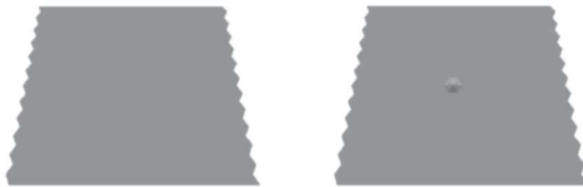
FIGURE 4.7: Visual stimulus presented to the subjects for measuring the Contrast Sensitivity Function in the case of flat shading. Left: the reference plane. Right: a vertex is displaced in the central area of the plane.
