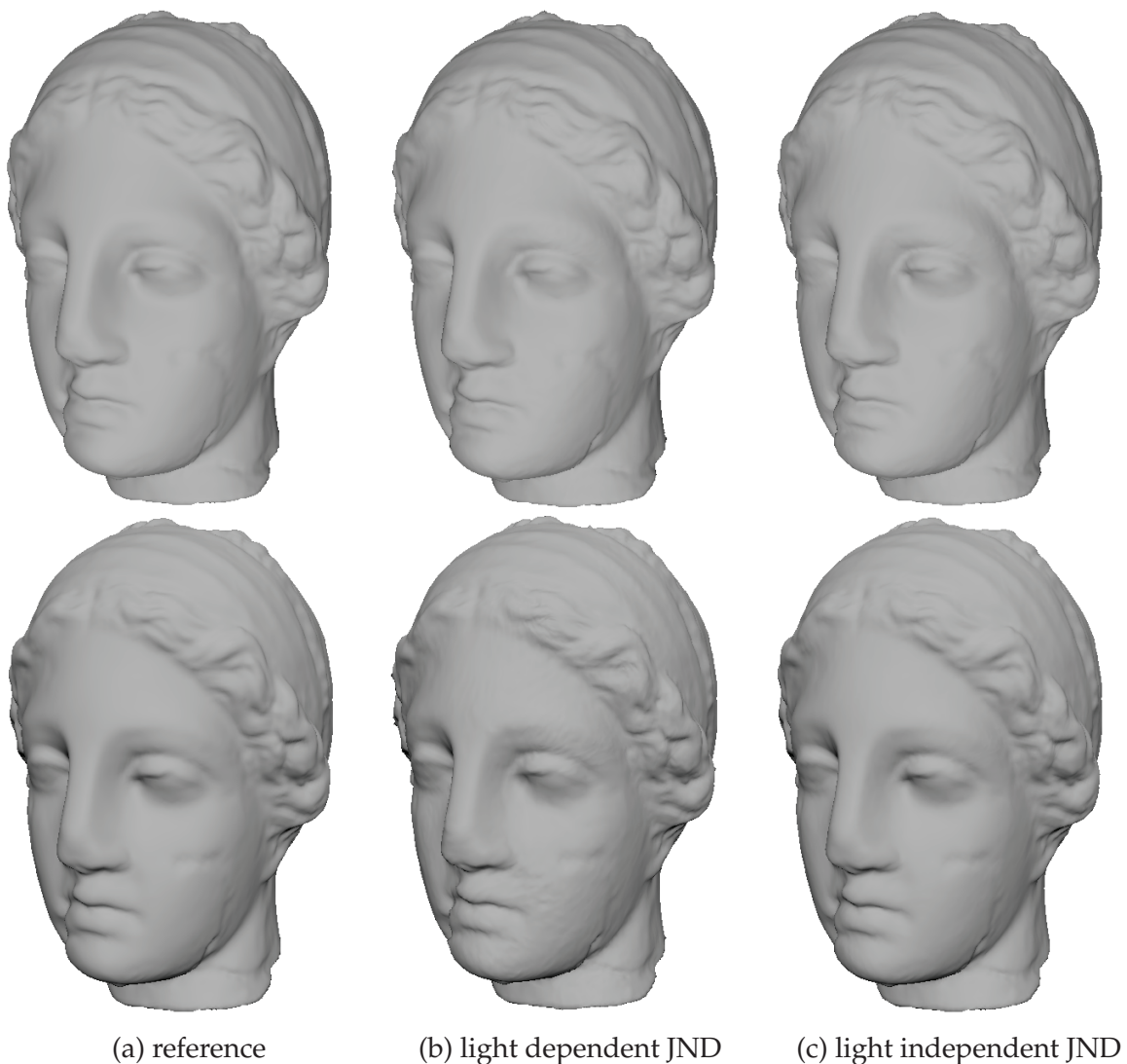
FIGURE 5.15: A vertex noise equivalent to the JND level computed in a light dependent mode might become visible when the light direction is altered between the two rows. This is not the case for light independent JND.
