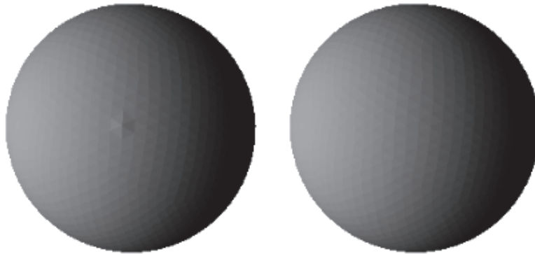
FIGURE 4.9: Visual stimulus for measuring threshold relative to the aspects of contrast masking in the case of flat shading. Left: a sphere approximated by an icosahedron subdivided 3 times from which a vertex is displaced. Right: the reference sphere.
