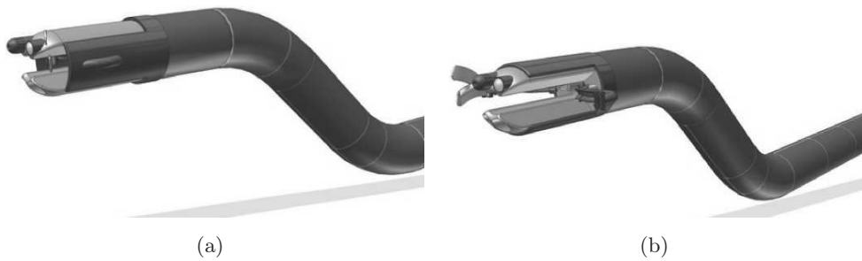
Figure 2.6: Transdouglass Endoscopic Device in the S-shape operational configuration. It is a 3 rigid links device with 4 working channels. Once positioned, the arms with the instruments are deployed as shown in (b). Moreover, the head of TED houses also a camera, a light and a dedicated channel for flushing and sucking (image: http://www.nesacademy.org ).
