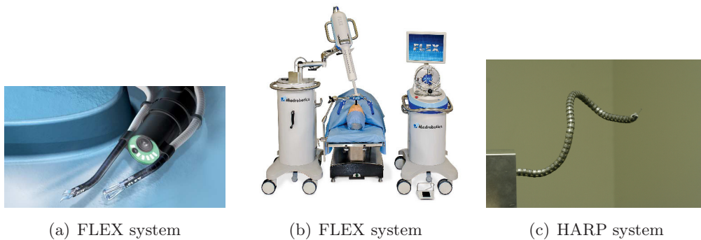
Figure 2.14: The FLEX system in (a) and (b) is composed by an endoscope and two working channels where specific instruments can be inserted (photos: medrobotics.com). The scope is self supporting and take inspiration from the HARP system in (c) (photo:carnegie mellon.)
