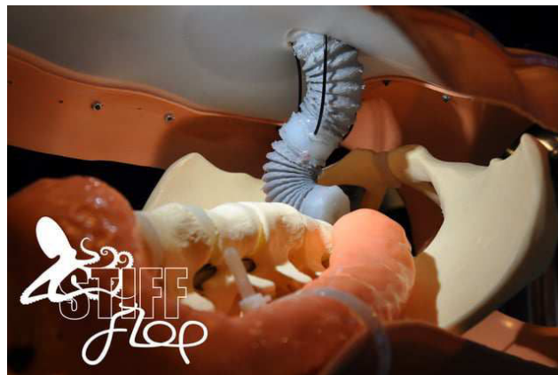
Figure 2.19: STIFF FLOP prototype. The robot can extend and compress and cable actuation allows to determine the shape of the two flexible sections (photo: National Museums Scotland - https://vimeo.com/97913172 ).
