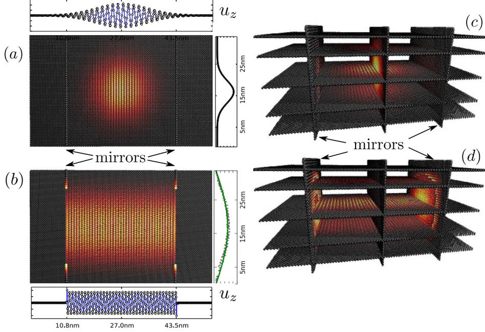
**Figure 4.6:** Atomic kinetic energy  $E_k$  in the nanocapacitor. Initial 3D phonon wave packet in a cutting plane (a) and in nanocapacitor (b). The final coherent standing-wave phonons with well defined wave-vectors  $\pm \mathbf{k}$  and wavelength  $\lambda_c$  confined in the capacitor in a cutting plane (c) and in 3D structure (d). Panels show the atomic displacements along the  $x$  and  $z$  directions in the initial WP (a) and in final standing wave (c).
