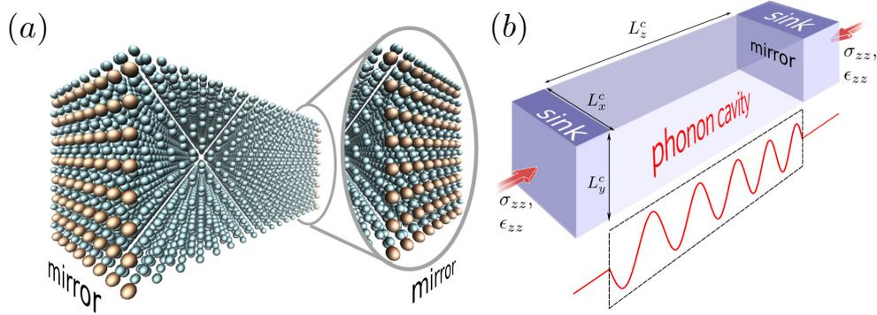
**Figure 4.1:** Silicon interference phonon capacitor composed of two interference phonon mirrors separated by a spacer. a) The atomistic view of the phonon capacitor and mirrors. The atoms in brown are Ge impurity atoms and the green ones are Si atoms of the host lattice. b) Phonon capacitor coupled to two heat sinks under the applied uniaxial stress  $\sigma_{zz}$ . The dimensions of the capacitor are  $L_x^c = L_y^c = 8$  nm and  $L_z^c = 35$  nm.
