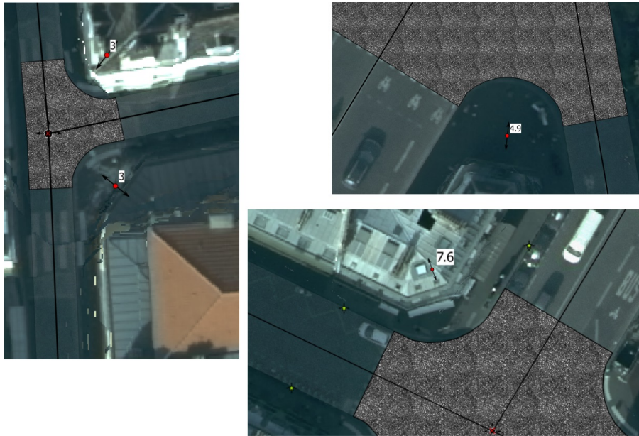
Figure 57: 3 different radius size (3m, 4.9m, 7.6 m) for streets of various importance, from real Paris data
