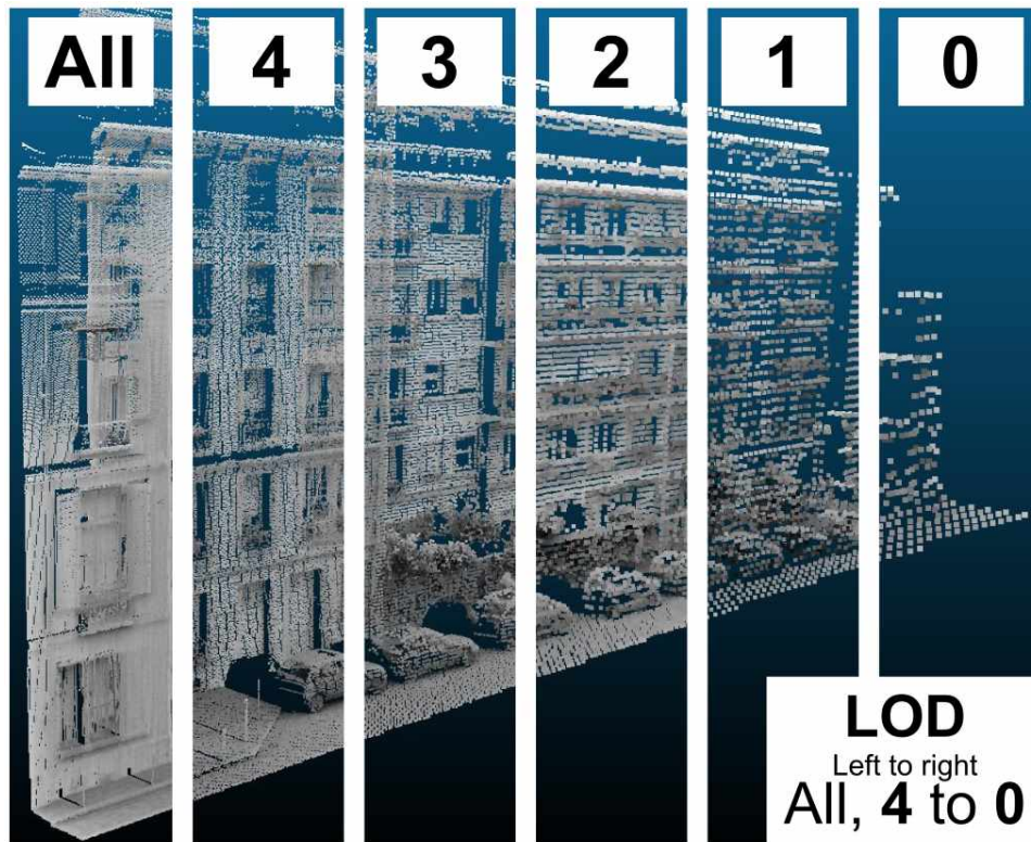
Figure 147: Schematic illustration of different LOD. Left to right, all points, then LOD 4 to 0. Visualized in cloud compare with ambient occlusion. Point size varies for better visual result.
