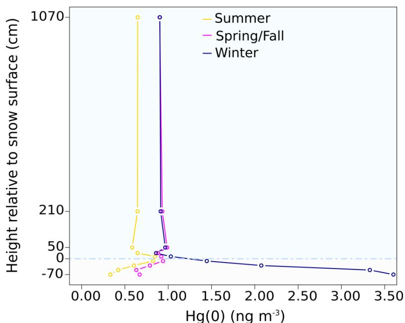
Figure 5-11: Mean Hg(0) concentration ( $\text{ng m}^{-3}$ ) measured at various heights above and below the snow surface (cm) at Concordia Station in summer (yellow), spring/fall (purple), and winter (dark blue). The horizontal light blue dashed line represents the snow surface.
