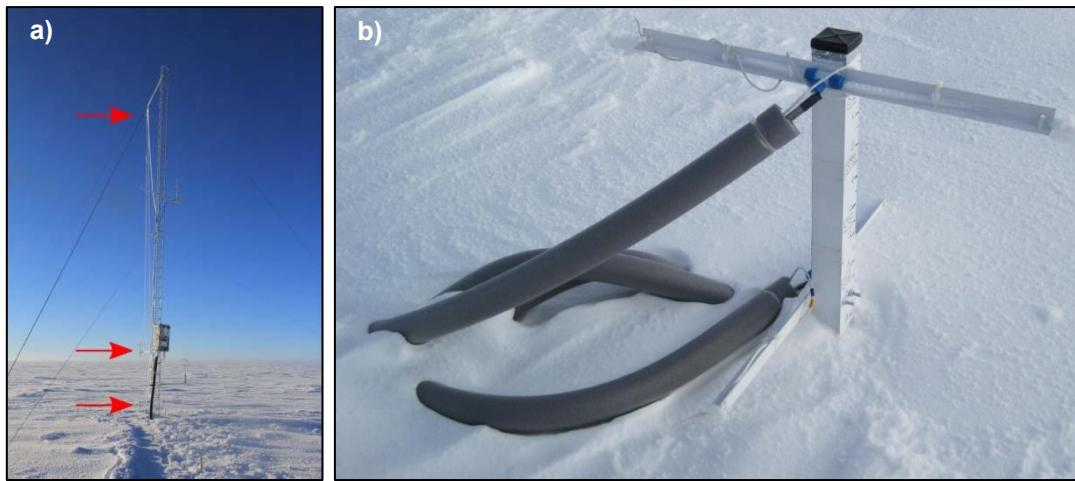
Figure 5-2: Photographs showing **a)** the meteorological tower with the three gas inlets (red arrows) at 1070 cm, 210 cm, and 25 cm above the snow surface (© B. Jourdain), and **b)** one of the snow towers with the two sampling inlets above the snowpack at 50 and 10 cm (© D. Helmig).
