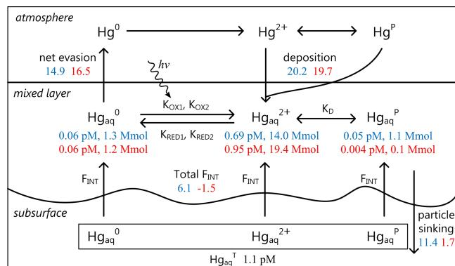
**Figure 6.** Global ocean mercury budget modeled by GEOS-Chem. Blue color indicates the reference simulation and red color the parameter inversion. Fluxes are in megamoles per year. Notations in this figure follow Soerensen et al. (2010b).  $F_{\text{INT}}$  denotes net fluxes from subsurface waters through entrainment/detrainment of the mixed layer and Ekman pumping.
