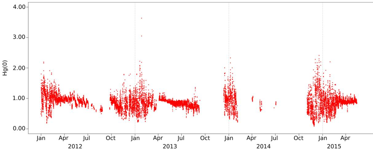
Figure 5-15: Hourly averaged Hg(0) concentrations (ng m<sup>-3</sup>) measured at DDU from January 2012 to May 2015. Missing data are due to instrument failure or QA/QC invalidation. Hg(0) concentrations were highly variable during the sunlit period as compared to wintertime (May–August) suggesting a photochemically induced reactivity in this period of the year.
