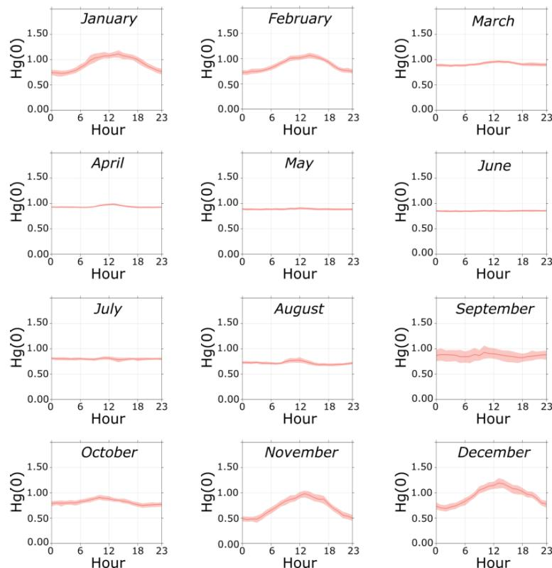
Figure 5-20: Monthly mean diurnal cycle of Hg(0) concentrations (in  $\text{ng m}^{-3}$ ) along with the 95 % confidence interval for the mean, calculated from all the data collected at DDU (January 2012-May 2015). Hours are in local time (UTC+10). Hg(0) concentrations exhibit a strong diurnal cycle in summer (November to February).
