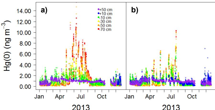
Figure 5-10: Annual variation of hourly averaged Hg(0) concentrations (in  $\text{ng m}^{-3}$ ) in the snow interstitial air collected at the various inlets of the two snow towers: **a)** snow tower #1, **b)** snow tower #2. Note that we regularly experienced technical problems on snow tower #2 leading to missing values.
