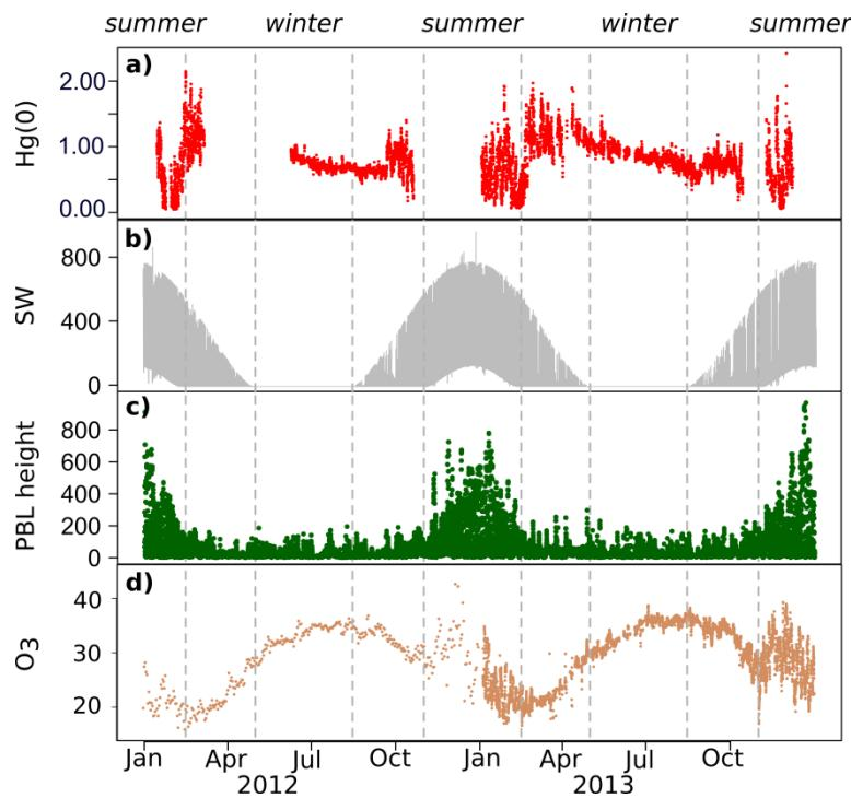
Figure 5-3: Annual variation in 2012 and 2013 of **a)** hourly averaged Hg(0) concentrations (in  $\text{ng m}^{-3}$ ) at 500 cm and 25 cm above the snow surface in 2012 and 2013, respectively, **b)** downwelling shortwave (SW) radiation (in  $\text{W m}^{-2}$ ), **c)** planetary boundary layer (PBL) height (in m), and **d)** ozone ( $\text{O}_3$ , daily mean in 2012 and hourly mean in 2013) mixing ratios (in ppbv). The vertical dashed lines represent seasonal boundaries.
