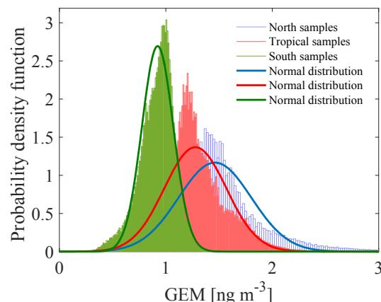
**Figure 4.** Probability density functions (PDFs) of the GEM data ( $\text{ng m}^{-3}$ ) for the northern, southern and tropical sample groups (dash dotted lines). Full lines the normal distribution fit of the samples.
