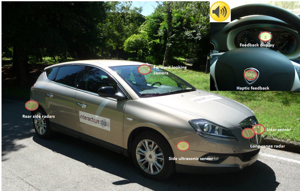
Figure 3.5: CRF demonstrator vehicle on Lancia Delta, with location of sensors and driver-interaction channels. Active safety belt is not shown.
