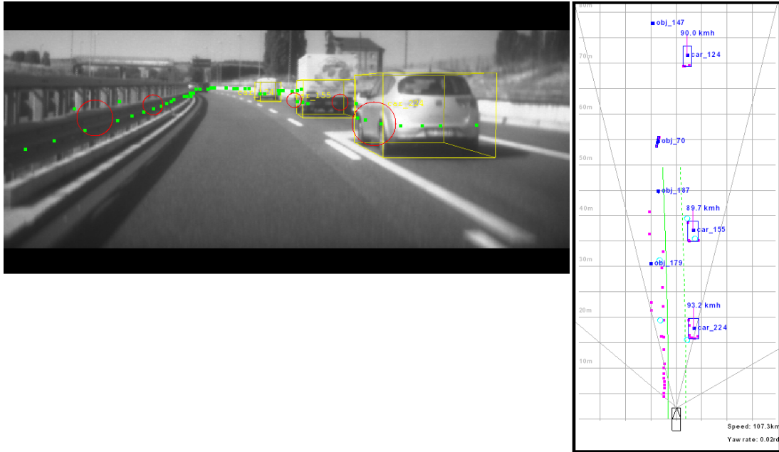
Figure 5.4: Results of the complete DATMO solution for a highway scenario. Vehicles at high speeds are detected. The left side of the figure shows the camera image and the identified moving objects. Yellow boxes represent moving objects, green dots represent lidar hits and red circles represent radar detections. The right side of each figure shows the top view of the scene presented in the image. Object classes are shown by tags close to each object.
