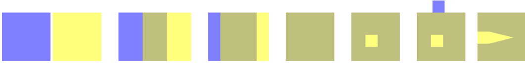
Figure 7.9: Example for dice coefficients from left to right : 0, 0.5, 0.75, 1, 2 * 15 / (16 + 15) = 0.968, 2 * 15 / (16 + 16) = 0.9375, 2 * 14 / (16 + 14) = 0.933
