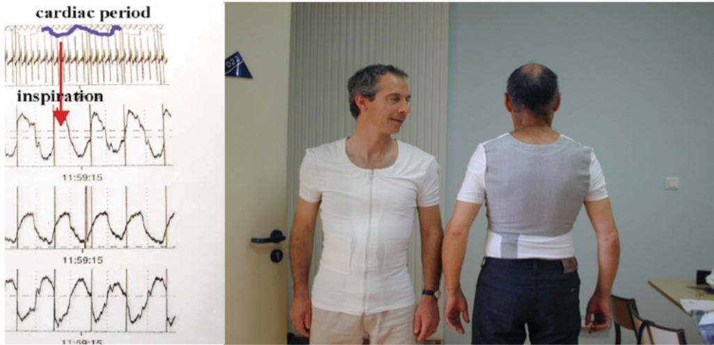
Fig. 4. Left: the sinus physiologic respiratory arrhythmia characterized by a decrease of the cardiac period during the inspiration. Right: the recording device giving the respiratory and cardiac rhythm from a smart tee-shirt containing a conductor whose impedance varies with chest expansion.
